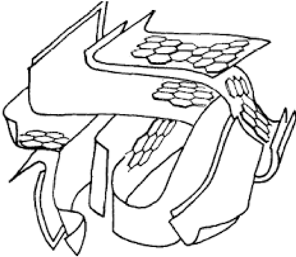
Figure 2: Structure of activated carbon (Stoeckli, 1990)
