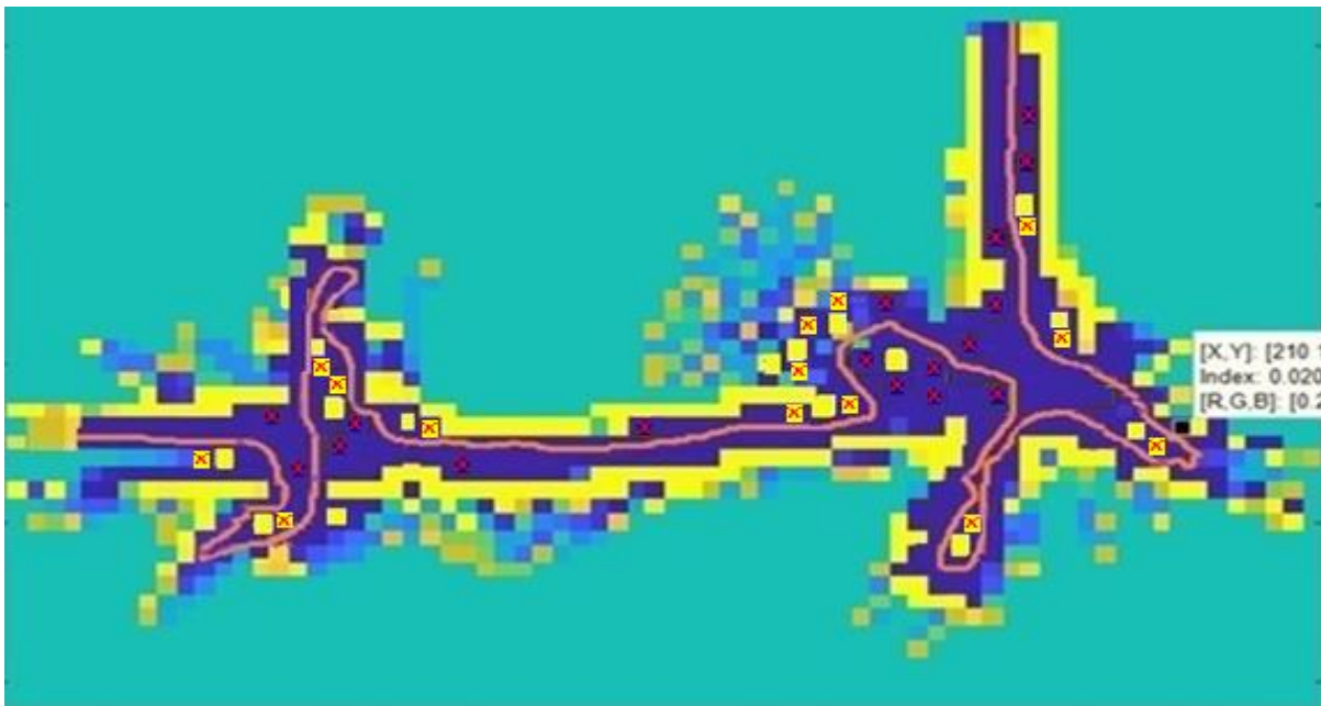
Figure 5-8b: Qualitative dynamic result for DIK-SLAM algorithm in 5% increase noise level
