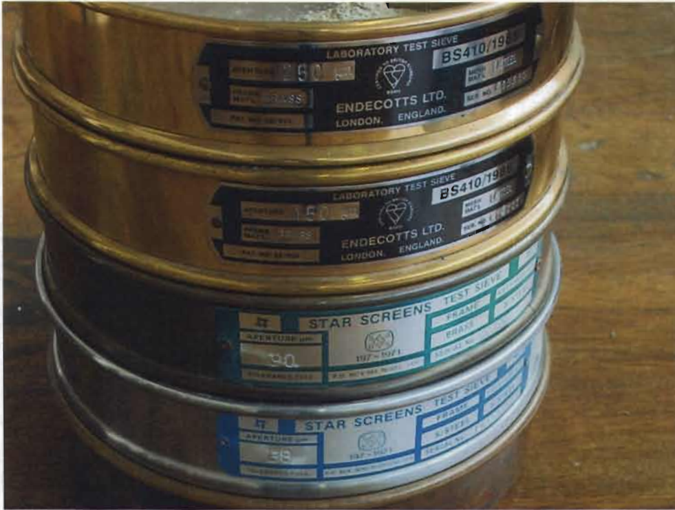
ANNEXURE 21 Particle screening sieves (250 \mu\text{m} , 150 \mu\text{m} , 90 \mu\text{m} and 38 \mu\text{m} ) placed on top of each other
