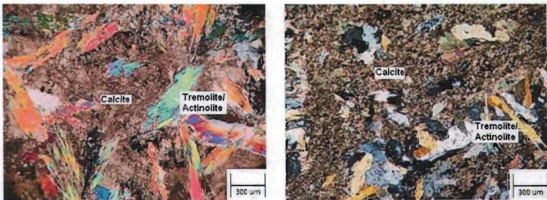
Figure 6.2: Photomicrographs of the untreated (left) and treated (right) JSB rock sample taken under cross-polarized light
