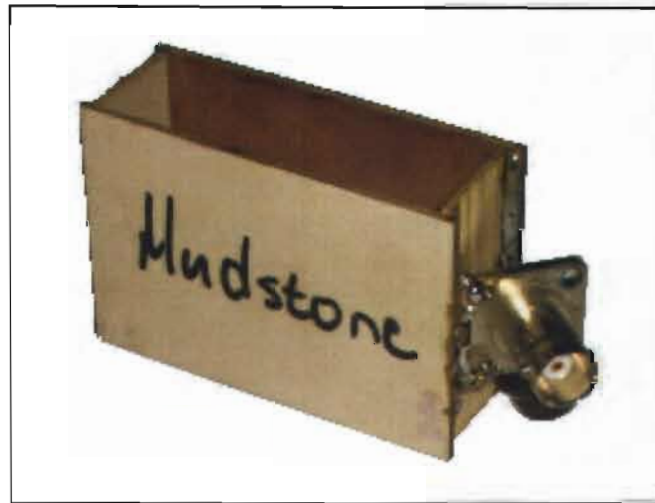
Figure 4.5: First prototype of the PPC with a BNC connector
