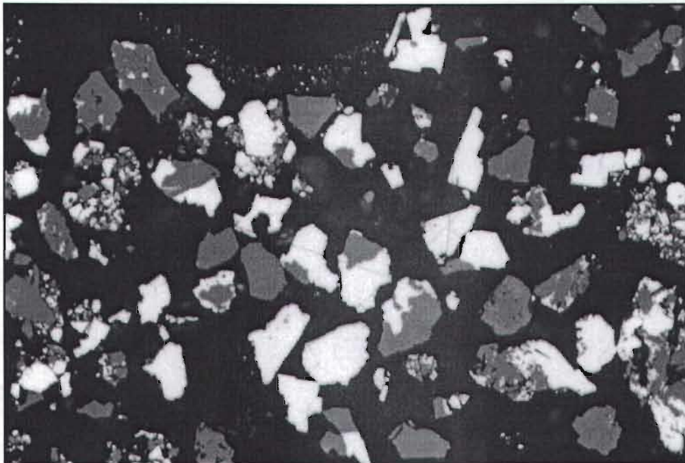
Figure 2.4: Photomicrograph of a concentrated lead-zinc ore, consisting of particles/fragments of the minerals galena and sphalerite - the degree of liberation in this sample is very variable with few liberated particles, but mostly middlings. The few liberated particles may only appear so in this particular section since the third dimension is not observable, and hence the term apparently liberated is used (Iyer and Duller 1998)
