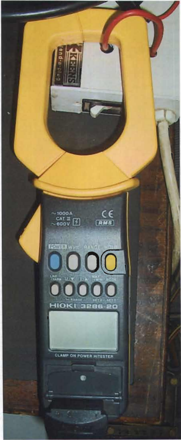
ANNEXURE 20 HIOKI 3286-20 clamp-on power meter used to measure the power consumption of the RF amplifiers and the swing-pot mill
