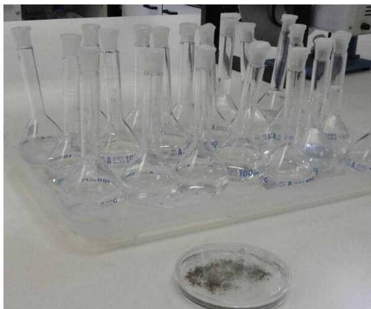
Figure 3.2: Apparatus for the dilution of nanoparticles using standard water
