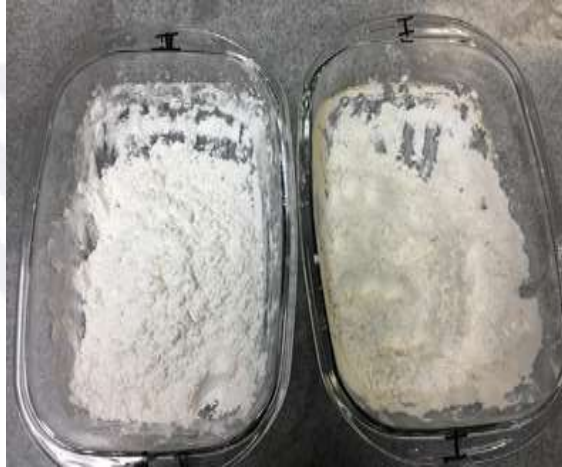
Cellulose nanocrystals modified with succinic anhydride and ethylenediaminetetraacetic acid
