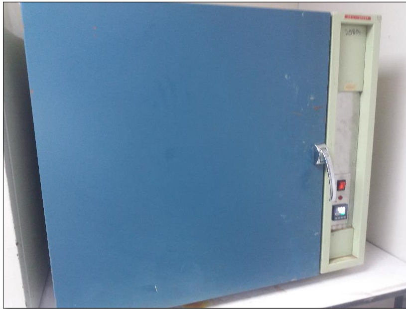
Figure 3-2 – Oven used for drying out fly samples
