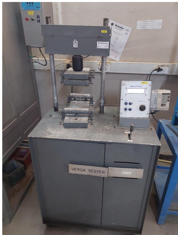
Figure 3-18 – Flexural Strength set up
