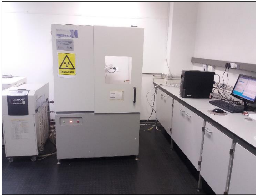
Figure 3-6 – XRD Diffraction analysis of fly ash sample on XRD-7000 Shimadzu
