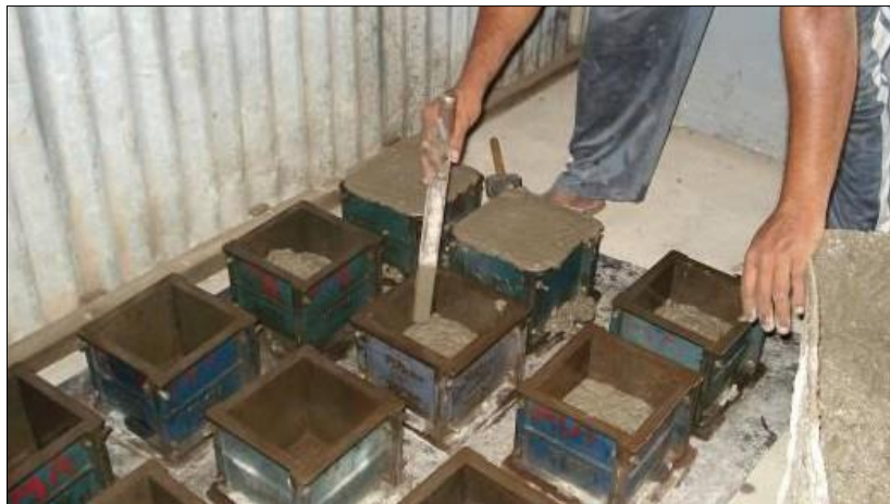
Figure 2-25 – Concrete cubes for compressive strength tests (Neyestani, 2011)
