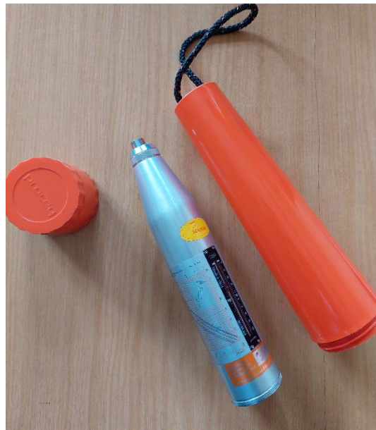
Figure 3-22 – Rebound Hammer Test
