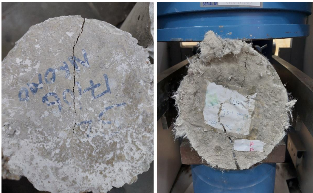
Figure 4-25 – Split Tensile Failure of Concrete Cylinder a) Unreinforced concrete b) FRCC
