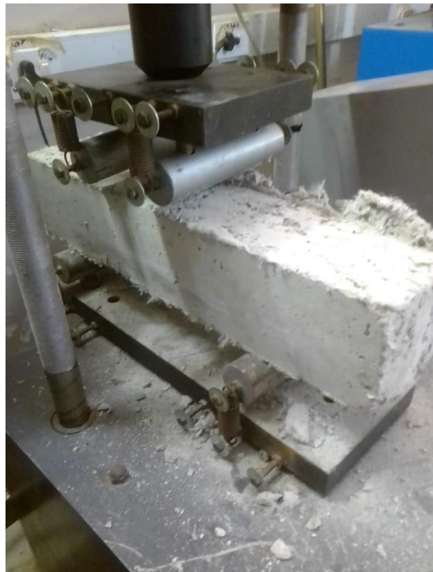
Figure 3-19 – Four Point flexural strength test setup
