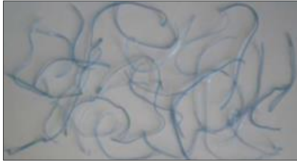
Figure 2-16 – Polyethylene Terephthalate tapes obtained from waste PET bottles (Wilinski, et al., 2016)
