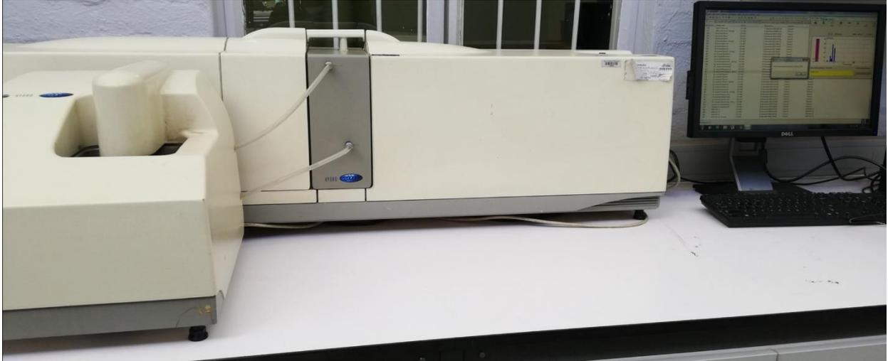
*Fig. 3.1: Malvern particle size analyser equipment*
