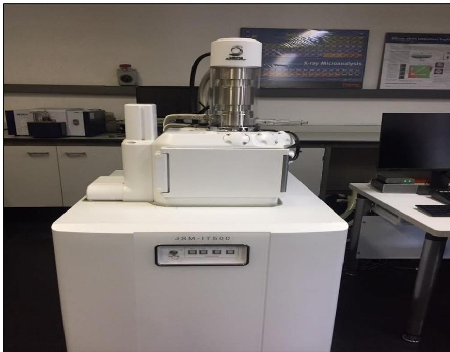
*Fig. 3.2: JEOL JSM-IT500 scanning electron microscopy (SEM) machine equipped with EDS*
