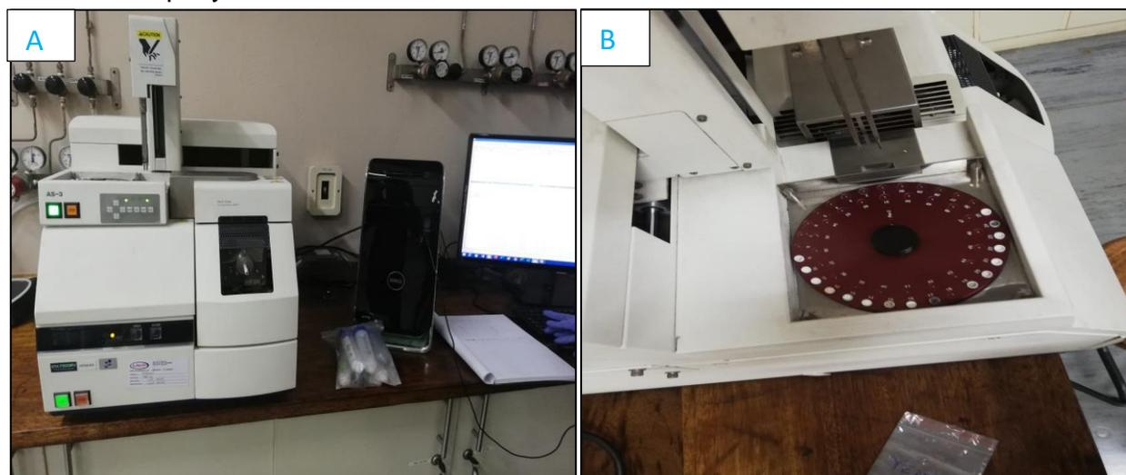
*Fig. 3.7 shows TGA/DSC equipment set up (A) STA7200RV TGA/DSC and (B) auto-sampler.*
