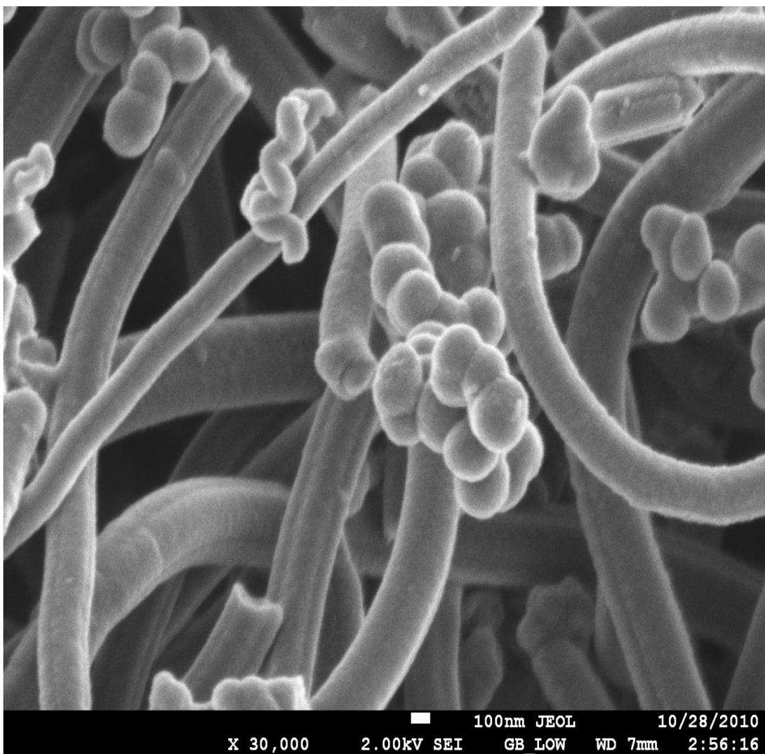
**Figure 4.19:** SEM image of carbon nanomaterial as-prepared from Co-Al
