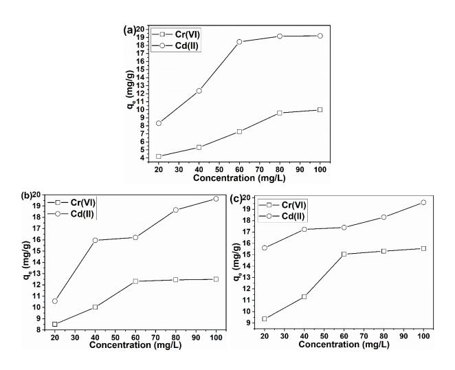
**Figure 31:** Initial concentration effect of (a) PBS, (b) KMBS and (c) H<sub>3</sub>BCS for the adsorption of Cr(VI) and Cd(II). [Conditions: adsorbent dosage (20 mg), volume of solution (20 ml), temperature of the system (298 K), agitation speed (300 rpm), pH of Cr(VI) solution was (1) and Cd(II) solution was (9)]
