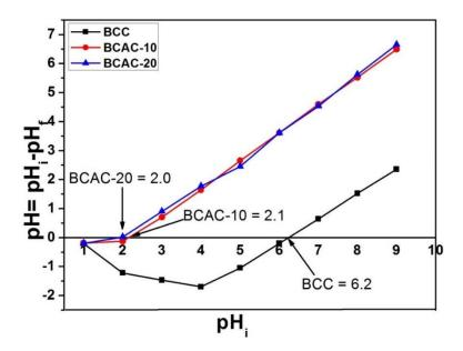
**Figure 50:** Point zero charge of adsorbents. [Experimental conditions: volume of solution (20 mL), time (720 min), adsorbent dosage (0.1 g), temperature (298 K), agitation rate (200 rpm), concentration (100 ppm)].
