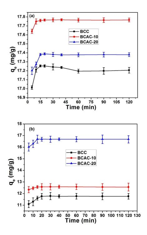
**Figure 47:** Time effect of (a) Pb(II) ions and (b) MB dye adsorption Onto BCC, BCAC-10 and BCAC-20 adsorbents. [Experimental conditions: volume of solution (20 mL), concentration (100 ppm), adsorbent dosage (0.1 g), temperature of the system (298 K), agitation rate (200 rpm), pH of solutions during Pb(II) ions and MB dye sorption (4.8)]
