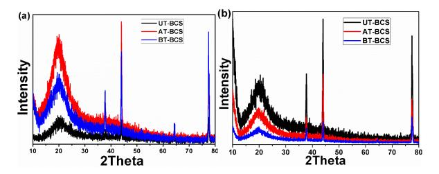
**Figure 19:** XRD spectra of UT-BCS, AT-BCS and BT-BCS; (a) before adsorption and (b) after adsorption.
