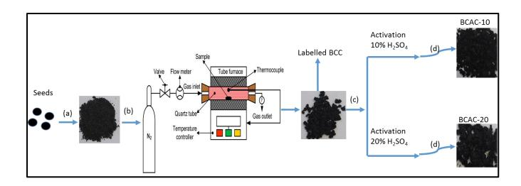
**Scheme 3**: Preparation of black cumin activated carbon (a) crushing (b) carbonization (c) activation (d) labelling
