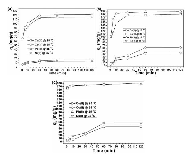
**Figure 22:** Time effect studies onto (a) UT-BCS, (b) AT-BCS and (c) BT-BCS for the adsorption of Cu(II), Co(II), Pb(II) and Ni(II)
