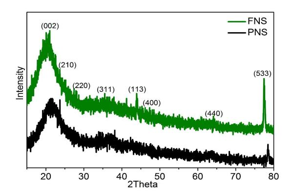
Figure 53: XRD spectra of FNS and PNS composites.
