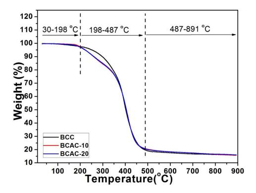
Figure 45: TGA of BCC, BCAC-10 and BCAC-20 adsorbents.
