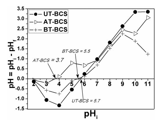
Figure 24: Point of zero charge of adsorbents
