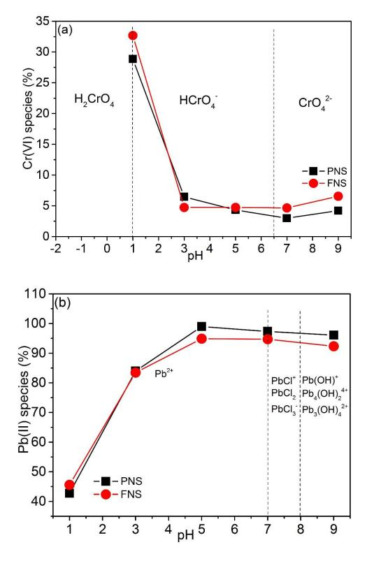
**Figure 55:** Speciation diagrams of **(a)** Cr(VI) and **(b)** Pb(II) ions Onto PNS and FNS composites at concentration of 100 mg/L at room temperature.
