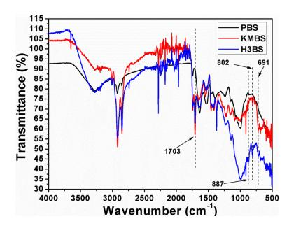
Figure 27: FTIR spectra of PBS, KMBS and H<sub>3</sub>BS
