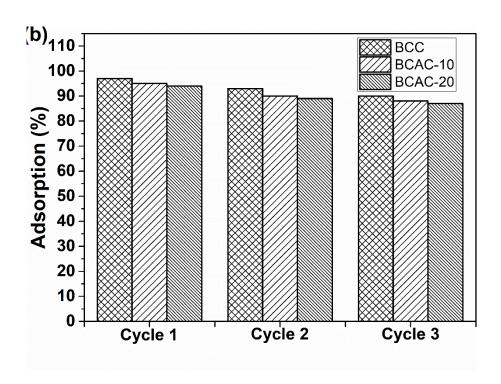
**Figure 51:** Reusability studies of the adsorption of (a) Pb(II) ions and (b) MB dye [Experimental conditions: volume of solution (20 mL), time (60 min), adsorbent dosage (0.1 g), temperature (298 K), agitation rate (200 rpm), concentration (100 ppm), pH(5)].
