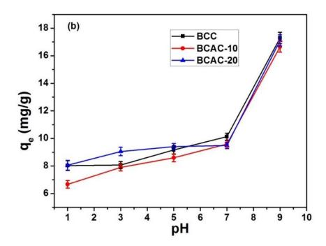
**Figure 49:** pH effect of (a) Pb(II) ions and (b) MB dye adsorption Onto BCC, BCAC-10 and BCAC-20 adsorbents. [Experimental conditions: volume of solution (20 mL), time (60 min), adsorbent dosage (0.1 g), temperature (298 K), agitation rate (200 rpm), concentration (100 ppm)]
