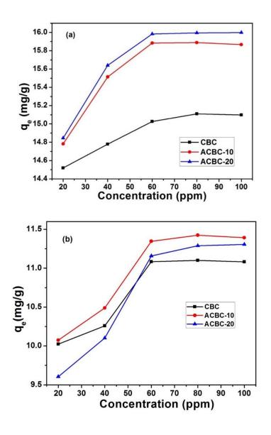
**Figure 37:** Concentration effect of (a) MB and (b) Cd(II) adsorption onto CBC, ACBC-10 and ACBC-20 adsorbents
