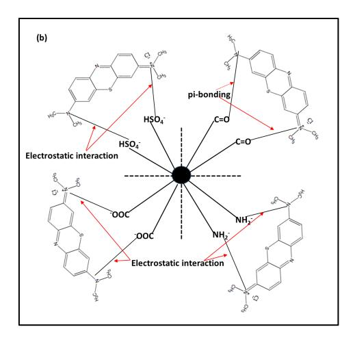
Scheme 4: Propose pathway for (a) Pb(II) ions and (b) MB dye interaction with the adsorbents.
