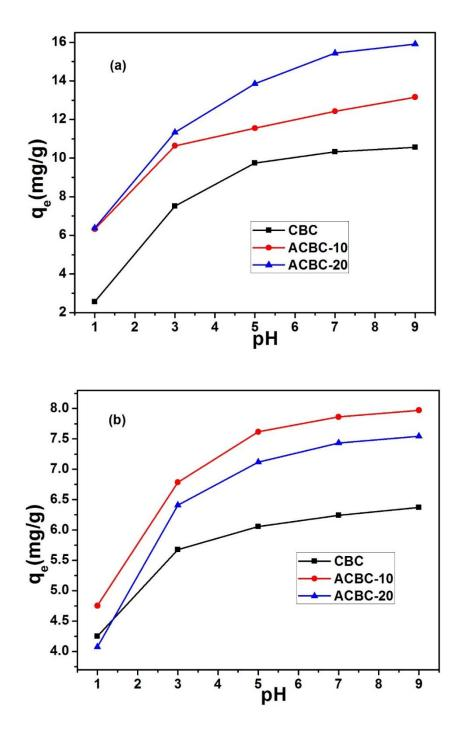
**Figure 40:** pH effect of (a) MB and (b) Cd(II) adsorption onto CBC, ACBC-10 and ACBC-20 adsorbents
