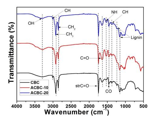
Figure 34: IR spectra of CBC, ACBC-10 and ACBC-20 adsorbents.
