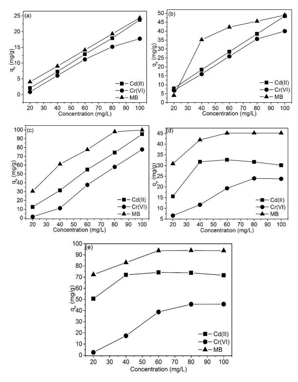
**Figure 63:** Effects of concentration on (a) PNS, (b) ANS, (c) CANS, (d) DNS and (e) CDNS for the adsorption of Cd(II), Cr(VI) and MB
