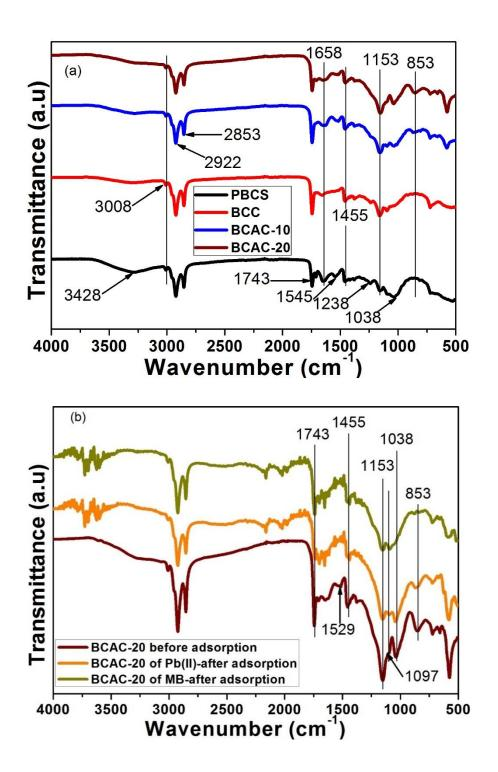
**Figure 43:** IR spectra of (a) PBCS, BCC, BCAC-10 and BCAC-20 adsorbents before adsorption, (b) BCAC-20 adsorbent before adsorption, BCAC-20 after adsorption for Pb(II) ions and BCAC-20 after adsorption MB dye.
