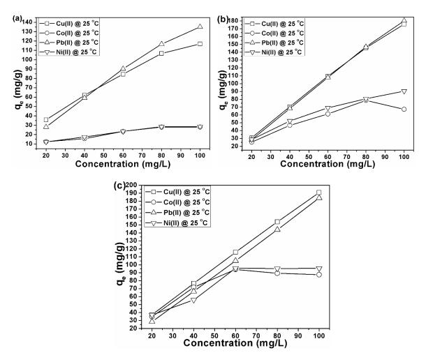
**Figure 20:** Concentration effect studies onto (a) UT-BCS, (b) AT-BCS and (c) BT-BCS for the adsorption of Cu(II), Co(II), Pb(II) and Ni(II)
