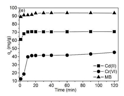
**Figure 62:** Effect of time on (a) PNS, (b) ANS, (c) CANS, (d) DNS and (e) CDNS for the adsorption of Cd(II), Cr(VI) and MB
