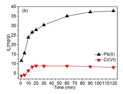
**Figure 57:** Time effect Onto (a) PNS and (b) FNS composites of Pb(II) ions and Cr(VI) sorption. [Experimental conditions: volume of solution (40 mL), concentration (100 ppm), adsorbent dosage (0.1 g), temperature of the system (298 K), agitation rate (200 rpm), pH of solutions during Pb(II) ions and Cr(VI) sorption (5)]
