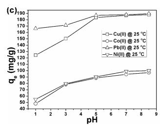
**Figure 23:** Effect of pH onto (a) UT-BCS, (b) AT-BCS and (c) BT-BCS for the adsorption of Cu(II), Co(II), Pb(II) and Ni(II)
