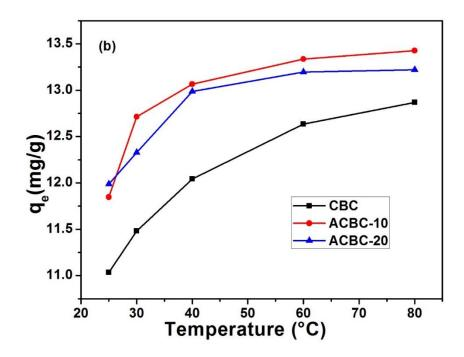
**Figure 39:** Temperature effect of (a) MB and (b) Cd(II) adsorption onto CBC, ACBC-10 and ACBC-20 adsorbents.
