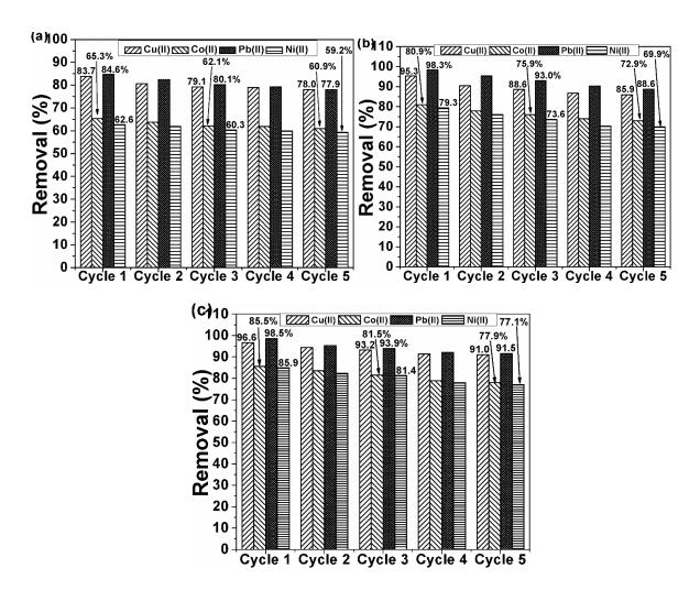
Figure 25: Reusability data of (a) UT-BCS (b) AT-BCS and (c) BT-BCS
