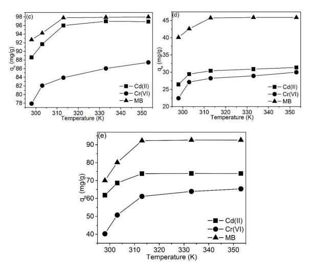
**Figure 64:** Effects of temperature on (a) PNS, (b) ANS, (c) CANS, (d) DNS and (e) CDNS for the adsorption of Cd(II), Cr(VI) and MB.
