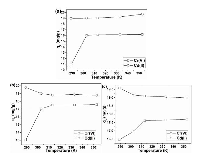
**Figure 32:** Temperature effect studies of (a) PBS, (b) KMBS and (c) H<sub>3</sub>BS for the adsorption of Cr(VI) and Cd(II) [Conditions: adsorbent dosage (20 mg), volume of solution (20 ml), agitation speed (300 rpm), pH of Cr(VI) solution was (1) and Cd(II) solution was (9)]
