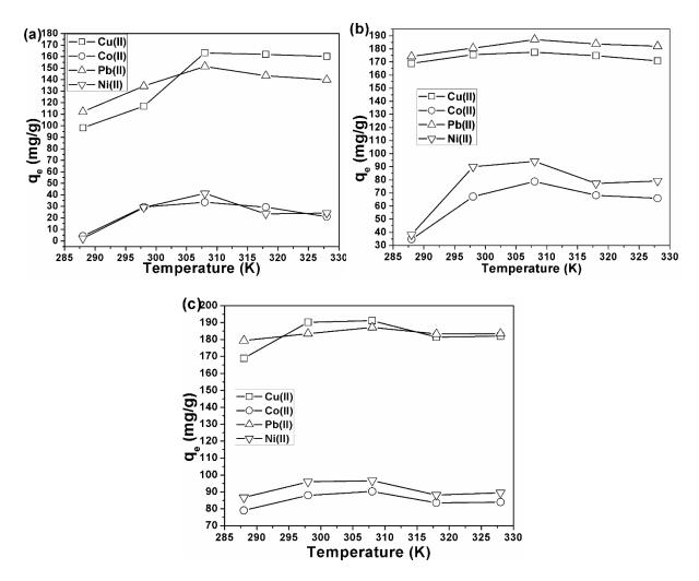
**Figure 21:** Temperature effect studies onto (a) UT-BCS, (b) AT-BCS and (c) BT-BCS for the adsorption of Cu(II), Co(II), Pb(II) and Ni(II)
