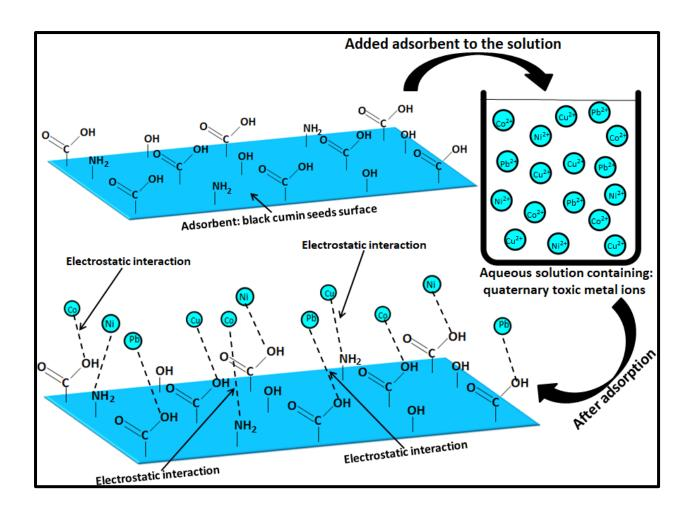
**Scheme 2:** Proposed adsorption mechanism of Cu(II), Pb(II), Ni(II) and Co(II) ions onto UT-BCS, AT-BCS and BT-BCS.
