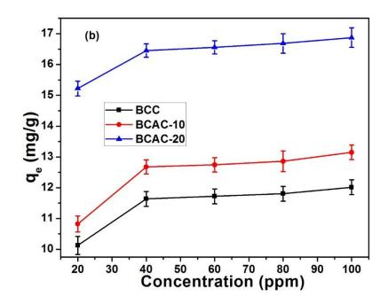
**Figure 46:** Concentration effect of (a) Pb(II) ions and (b) MB dye adsorption Onto BCC, BCAC-10 and BCAC-20 adsorbents [Experimental conditions: volume of solution (20 mL), time (60 min), adsorbent dosage (0.1 g), temperature of the system (298 K), agitation rate (200 rpm), pH of solutions during Pb(II) ions and MB dye sorption (4.8)]
