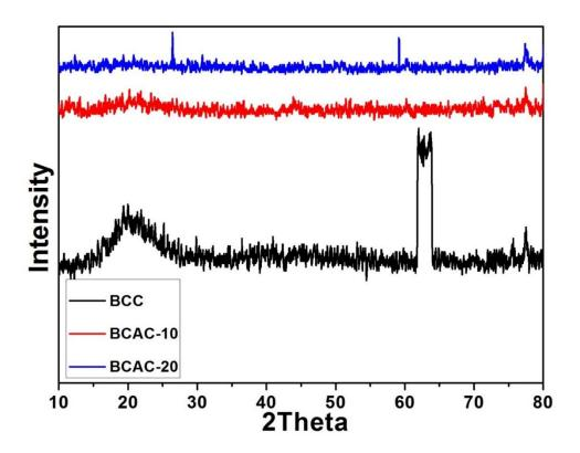
Figure 44: XRD spectra of BCC, BCAC-10 and BCAC-20 adsorbents.
