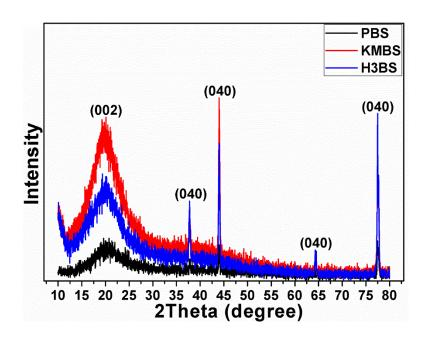
Figure 28: XRD diffraction of PBS, KMBS and H<sub>3</sub>BS
