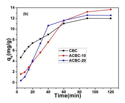
**Figure 38**: Time effect of (a) MB and (b) Cd(II)) adsorption onto CBC, ACBC-10 and ACBC-20 adsorbents
