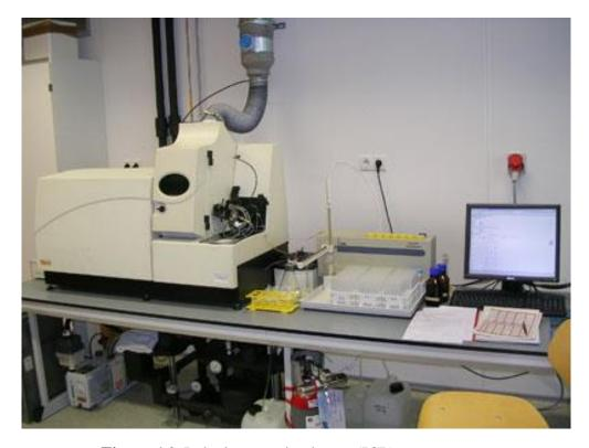
Figure 16: Inducive couple plasma (ICP) spectrometer
