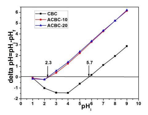
**Figure 41:** Point zero charge of MB and Cd(II) onto CBC, ACBC-10 and ACBC-20 adsorbents
