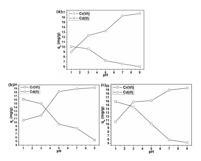
**Figure 29:** pH effect plots of (a) PBS, (b) KMBS and (c) H<sub>3</sub>BS for the adsorption of Cr(VI) and Cd(II). [Conditions: adsorbent dosage (20 mg), volume of solution (20 ml), concentration of solution (100 m/L), temperature of the system (298 K), agitation speed (300 rpm) and agitation time (120 min)]
