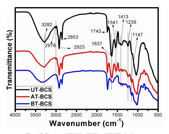
Figure 18: IR spectra of UT-BCS, AT-BCS and BT-BCS adsorbents
