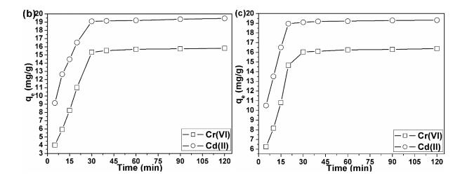
**Figure 30:** Contact time effect plots (a) PBS, (b) KMBS and (c) H<sub>3</sub>BCS for the adsorption of Cr(VI) and Cd(II). [Conditions: adsorbent dosage (20 mg), volume of solution (20 ml), concentration of solution (100 m/L), temperature of the system (298 K), agitation speed (300 rpm), pH of Cr(VI) solution was (1) and Cd(II) solution was (9)]
