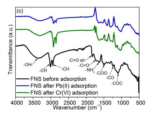
**Figure 52:** IR spectra of (a) PNS and FNS composites before adsorption, (b) PNS composite before and after adsorption and (c) FNS composite before and after adsorption of Pb(II) ions and Cr(VI).
