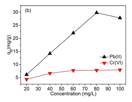
**Figure 56:** Concentration effect Onto (a) PNS and (b) FNS composites for Pb(II) ions and Cr(VI) sorption. [Experimental conditions: volume of solution (40 mL), time (60 min), adsorbent dosage (0.1 g), temperature of the system (298 K), agitation rate (200 rpm), pH of solutions during Pb(II) ions and Cr(VI) sorption (5.0)]
