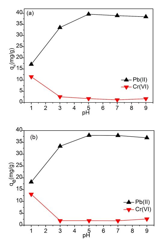
**Figure 54:** pH effect Onto (a) PNS and (b) FNS composites for Pb(II) ions and Cr(VI) sorption. [Experimental conditions: volume of solution (40 mL), time (60 min), adsorbent dosage (0.1 g), temperature (298 K), agitation rate (200 rpm), concentration (100 ppm)]
