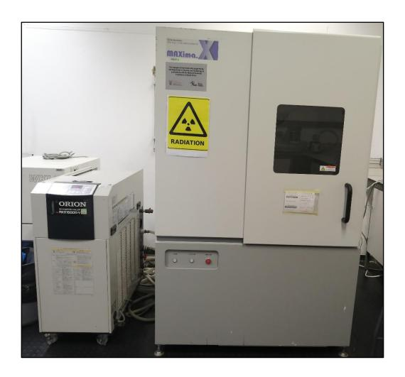
**Figure 6:** X-ray diffractometer (XRD)
