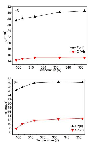
**Figure 58:** Temperature effect **(a)** PNS and **(b)** FNS composites of Pb(II) ions and Cr(VI) sorption. [Experimental conditions: volume of solution (40 mL), time (60 min), adsorbent dosage (0.1 g), concentration (100 ppm), agitation rate (200 rpm), pH of solutions during Pb(II) ions and Cr(VI) sorption (5)]
