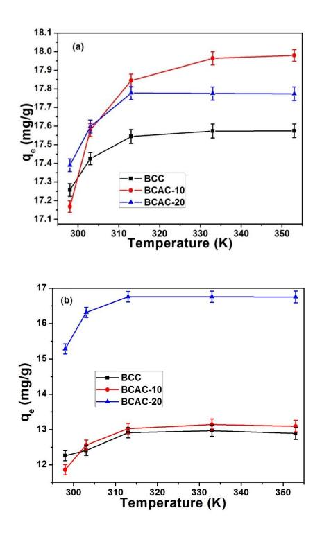
**Figure 48:** Temperature effect of (a) Pb(II) ions and (b) MB dye adsorption Onto BCC, BCAC-10 and BCAC-20 adsorbents. [Experimental conditions: volume of solution (20 mL), time (60 min), adsorbent dosage (0.1 g), concentration (100 ppm), agitation rate (200 rpm), pH of solutions during Pb(II) ions and MB dye sorption (4.8)]
