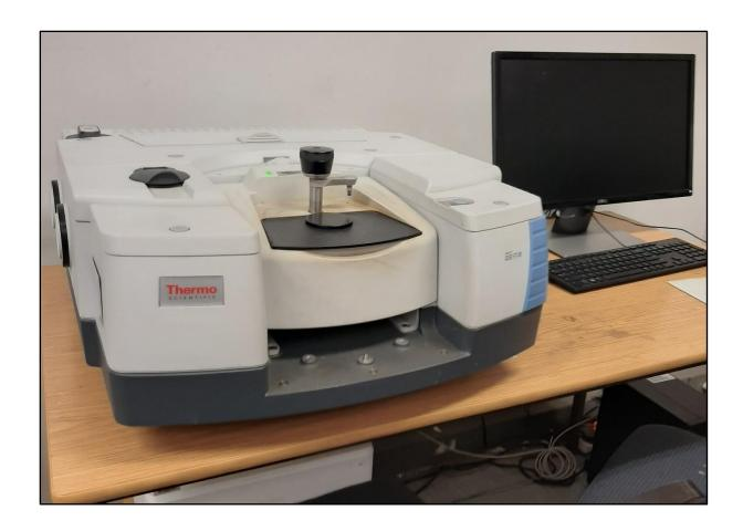
Figure 7: Fourier transformed infrared (FTIR) spectrophotometer
