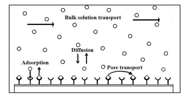
**Figure 1**: Schematic presentation of the adsorption process (Moon & Palaniandy, 2019)
