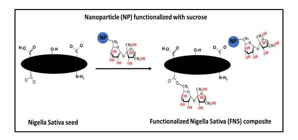
**Scheme 5:** Schematic of sucrose functionalized *Nigella Sativa* seeds (FNS) preparation **8.4 Batch adsorption studies**
