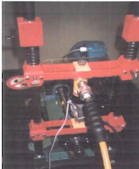
Figure 3.7: Test Bearing Loading Mechanism with Load Cell and Accelerometer
