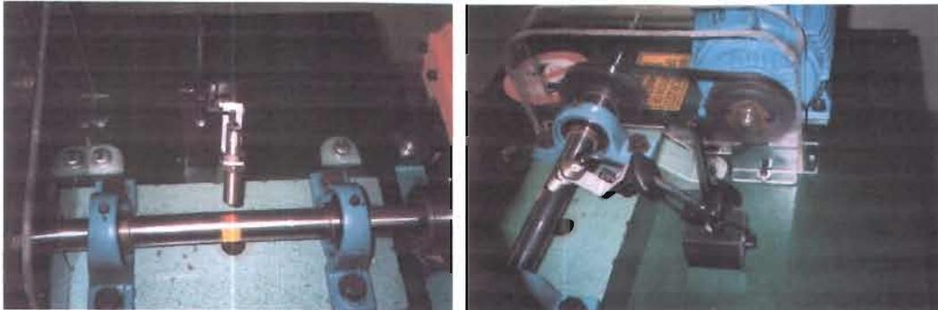
Figure 3.5: Test Bearing Shaft and V-Belt Drive System
