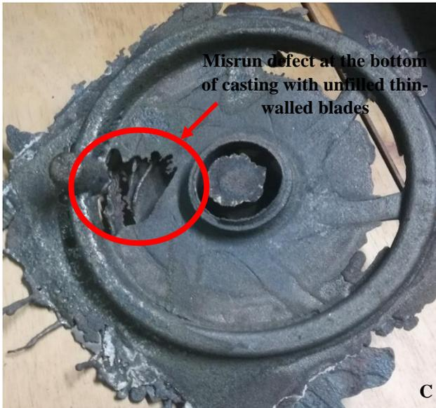
Figure 4. 53A, 4.53B & 4.53C: Misrun defect on an austenitic stainless-steel pump impeller cast at 1497°C.
