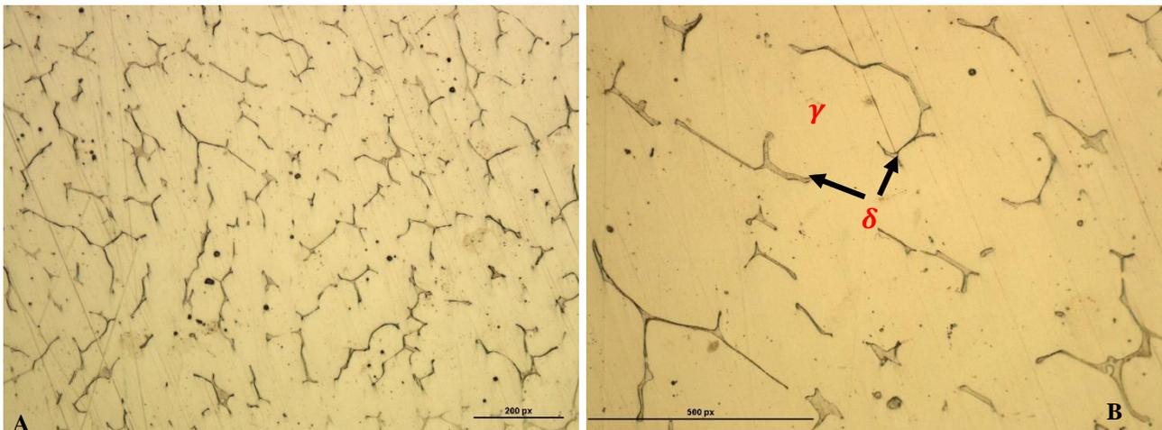
Figure 4. 54A and 4.54B: As cast microstructure of an austenitic stainless steel pump impeller at 20X (A) and 50X (B) magnification.
