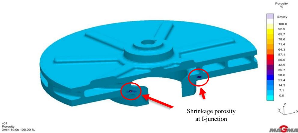
Figure 4. 52: Porosity results of design VX04 after solidification
