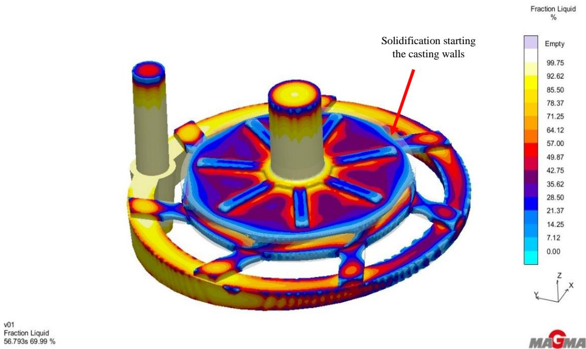
Figure 4. 59: Solidification simulation of design VX05 after 30% solid in 57 seconds
