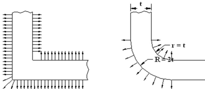
Figure 2. 8: Direction of heat transfer from solidifying metal to mould.
