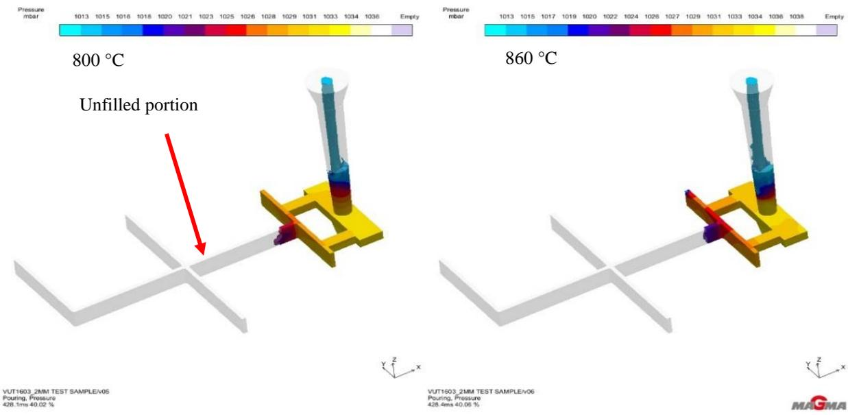
Figure 4. 3A: A representation of the metal pressure after 430 milliseconds of 2 mm test sample at 700 °C to 860 °C pouring temperature. The blue colour represents the lowest pressure of poured metal, red representing the average pressure, pale yellow indicating highest pressure and white shows unfilled portion.
