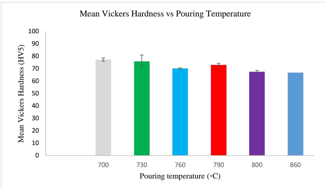
Figure 4. 9: Vickers hardness vs pouring temperature
