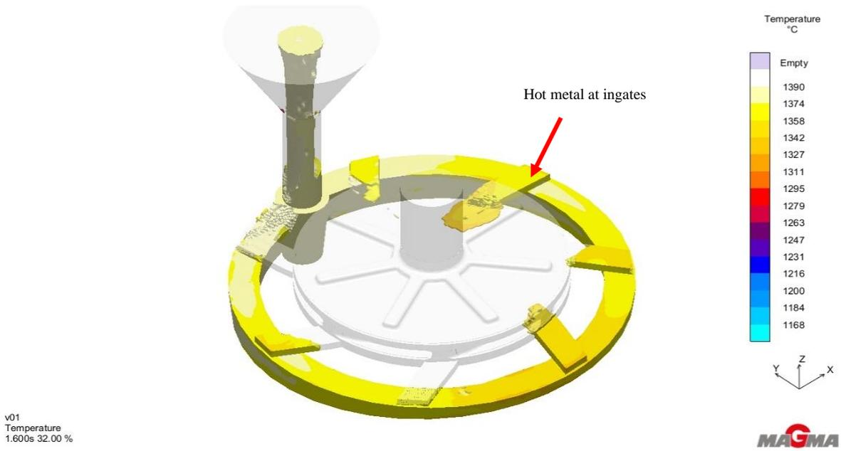
Figure 4. 56: Filling simulation of design VX05 at 32% filling ability after 1.6 seconds
