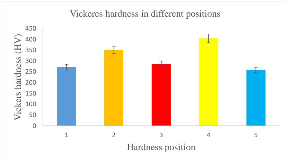
Figure 4. 37: Vickers hardness results of an as cast austenitic stainless steel at different positions
