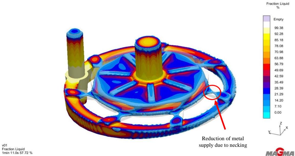
Figure 4. 60: Solidification simulation of design VX05 after 42.3% solid in 71 seconds
