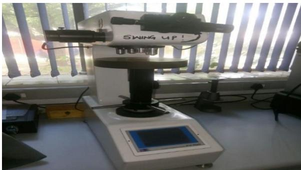
Figure 3. 8: Vickers hardness machine (FV700)
