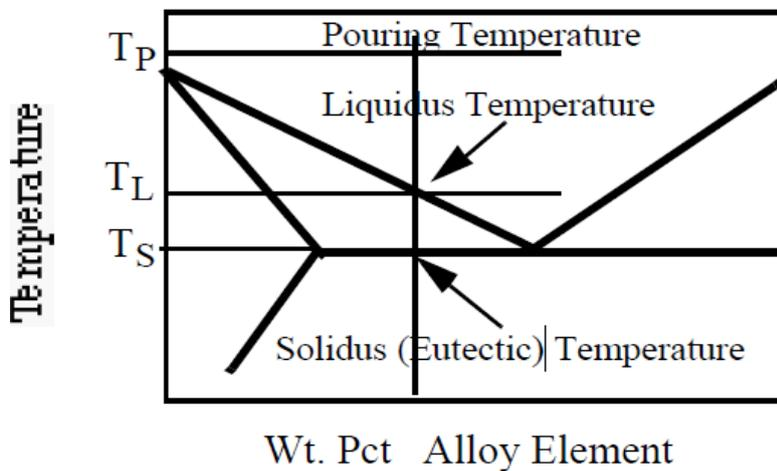
Figure 2. 3: A schematic representation of pouring temperature
