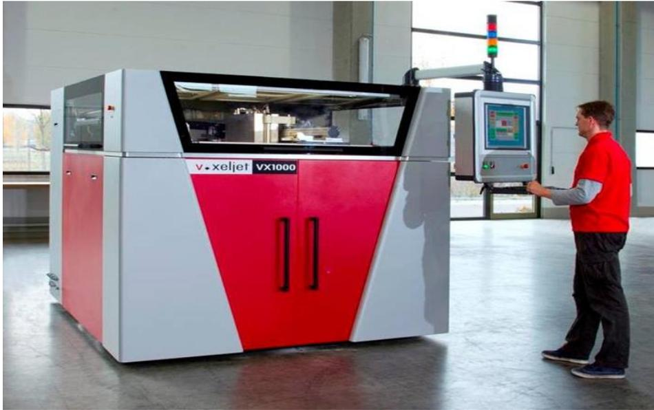
Figure 2. 15: Overview of Voxeljet VX1000 3D printer
