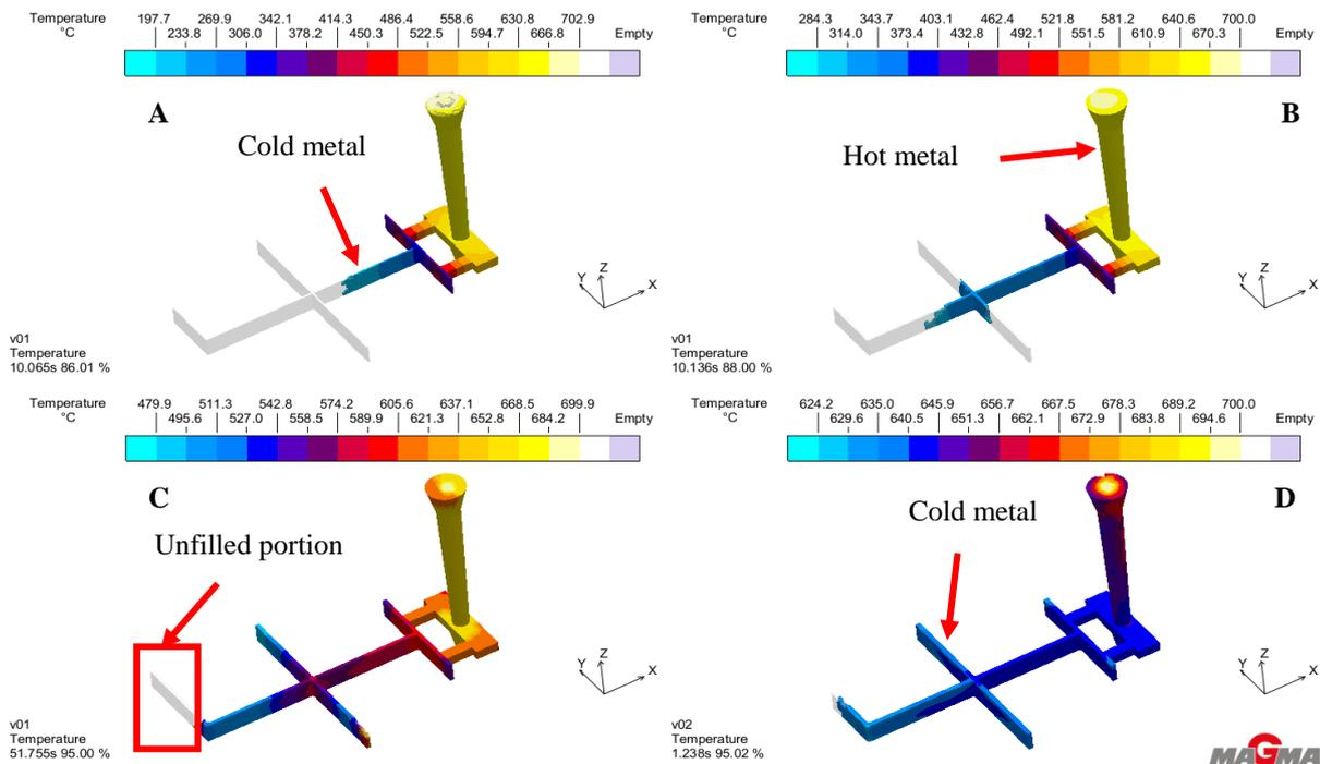
Figure 4. 10: Filling ability of 1 mm (A), 1.5 mm (B), 2 mm (C) and 2.5 mm (D) at 700 °C pouring temperature.
