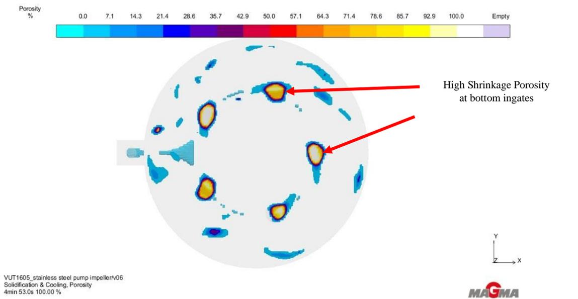
Figure 4. 19: Top-view showing shrinkage porosity at bottom ingates
