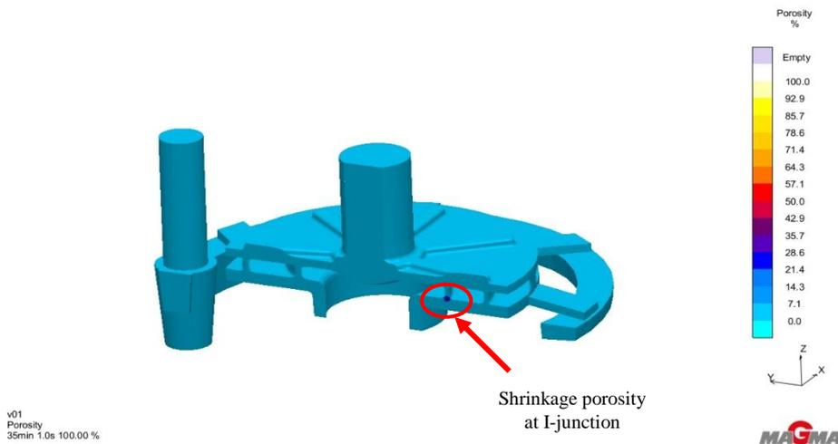
Figure 4. 63: Porosity results of design VX05 after 2100 seconds solidification
