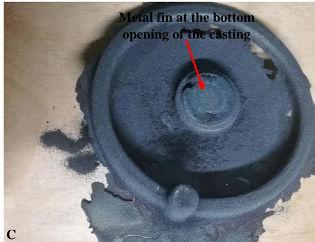
Figure 4. 64A, 4.64B & 4.64C: Completely-filled nodular cast iron pump impeller with minor slag entrapment at the top surface of the casting and the feeder and metal fin at parting line.
