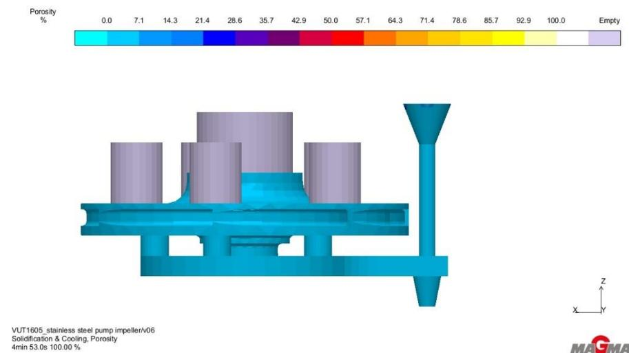
Figure 4. 16: A schematic view of design VX 01 runner system
