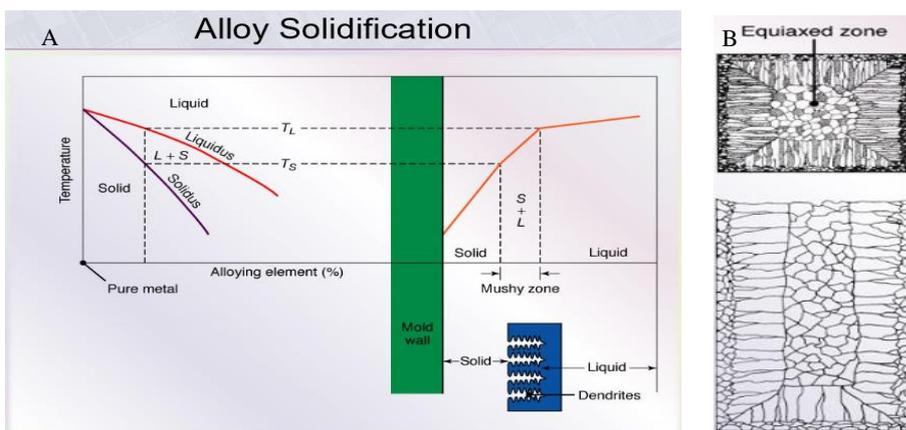
Figure 2. 11: Schematic illustration of alloy solidification (A) and alloy microstructure (B)
