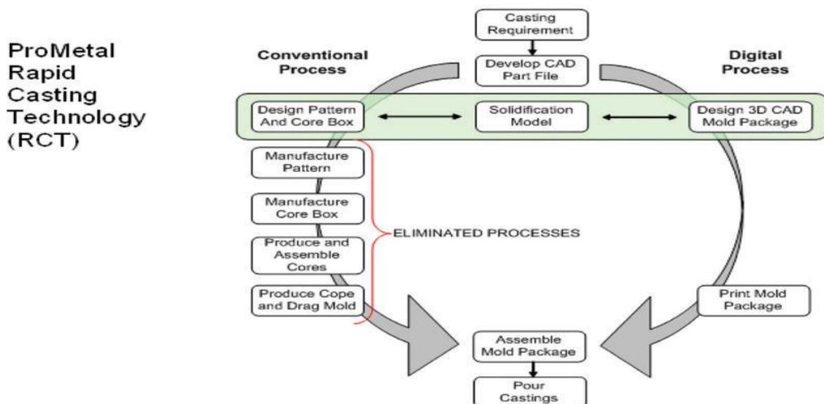
Figure 2. 16: Conventional vs digital mould making process.
