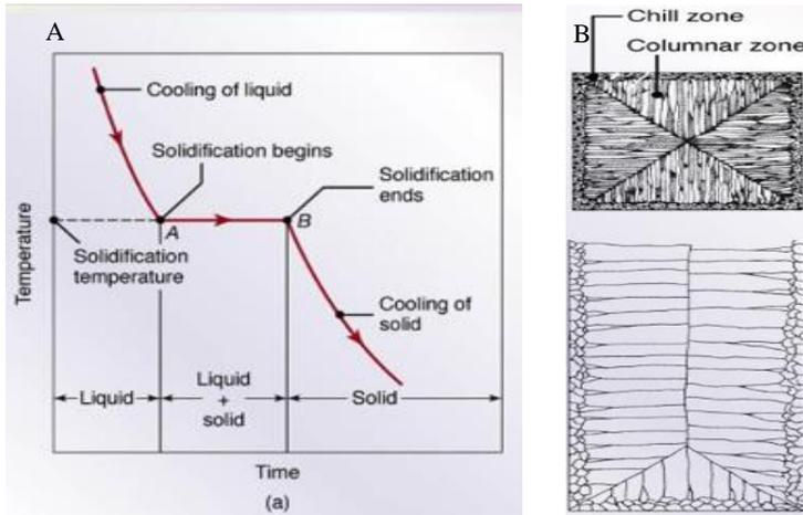
Figure 2. 10: Temperature as a function of time for pure metal (A) and microstructure of metal (B).
