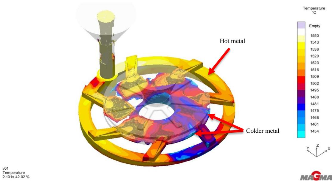
Figure 4. 48: Filling simulation of design VX04 at 42% filling ability
