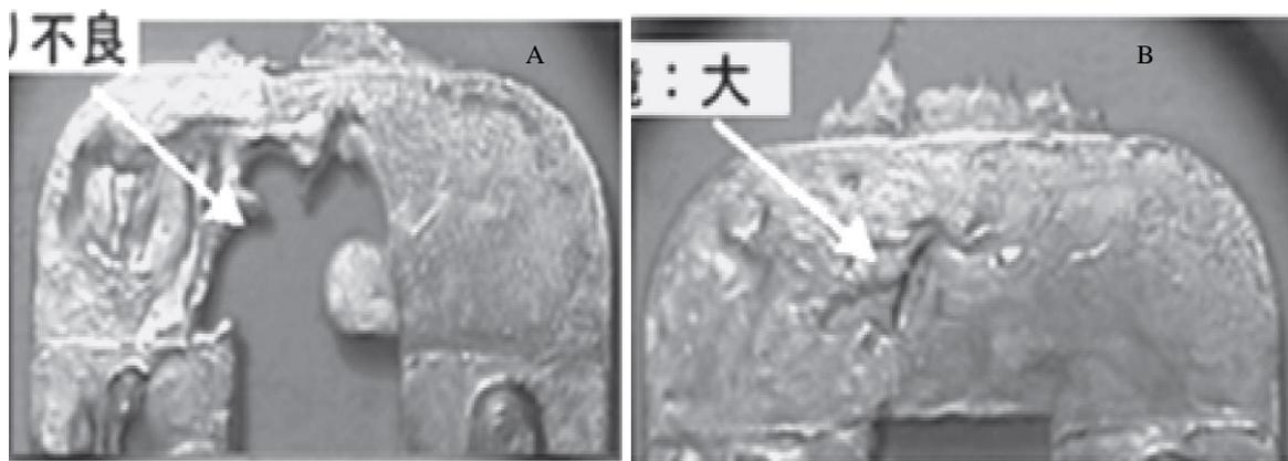
Figure 2. 2: Misrun (A) and cold-shut (B) defect
