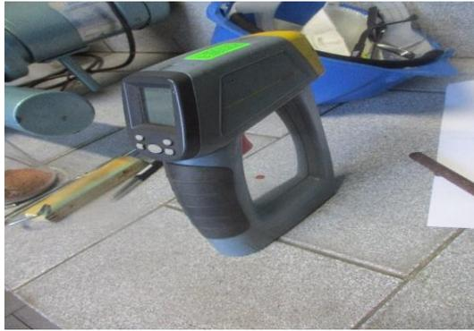
Figure 3. 4: Laser pyrometer
