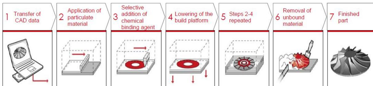
Figure 2. 17: Voxeljet VX1000 step by step printing process
