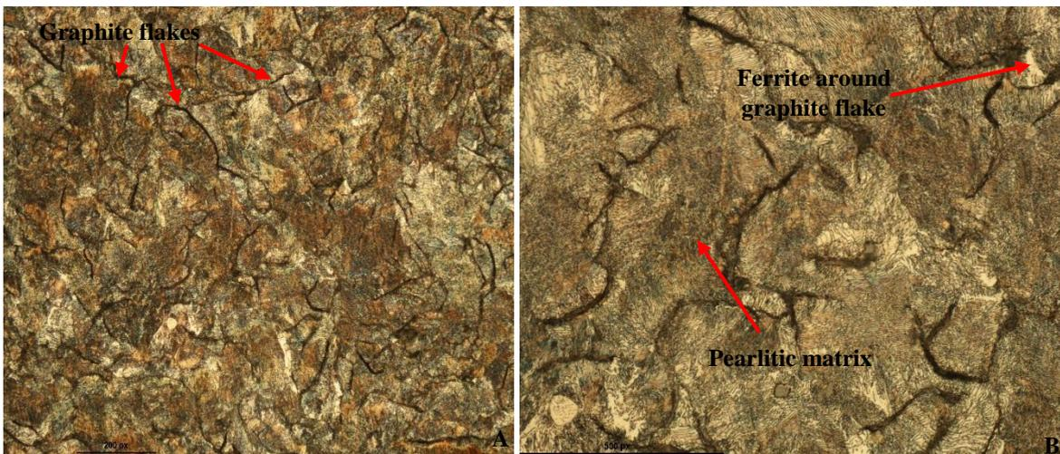
Figure 4. 65A & 4.65B: As cast microstructure of a nodular cast iron pump impeller at 20X (A) and 50X (B) magnification
