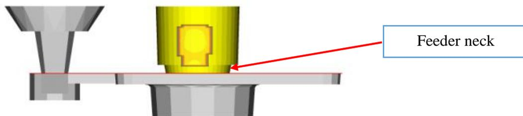
Figure 2. 7: Representation of feeder neck in a casting.
