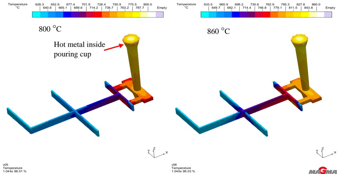
Figure 4. 1: Schematic representation of the simulation results showing the degree of molten metal filling at progressively increasing temperatures. The blue colour represents solidified metal, white represents unfilled portion and pale yellow represents hot metal.
