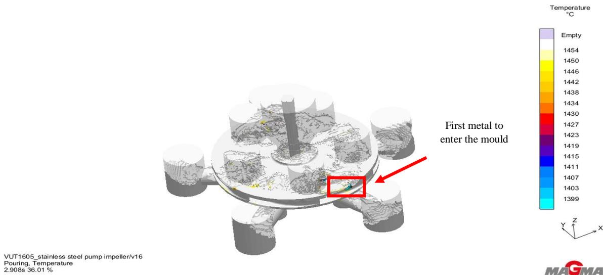
Figure 4. 31: Filling simulation of casting after 2.9 seconds
