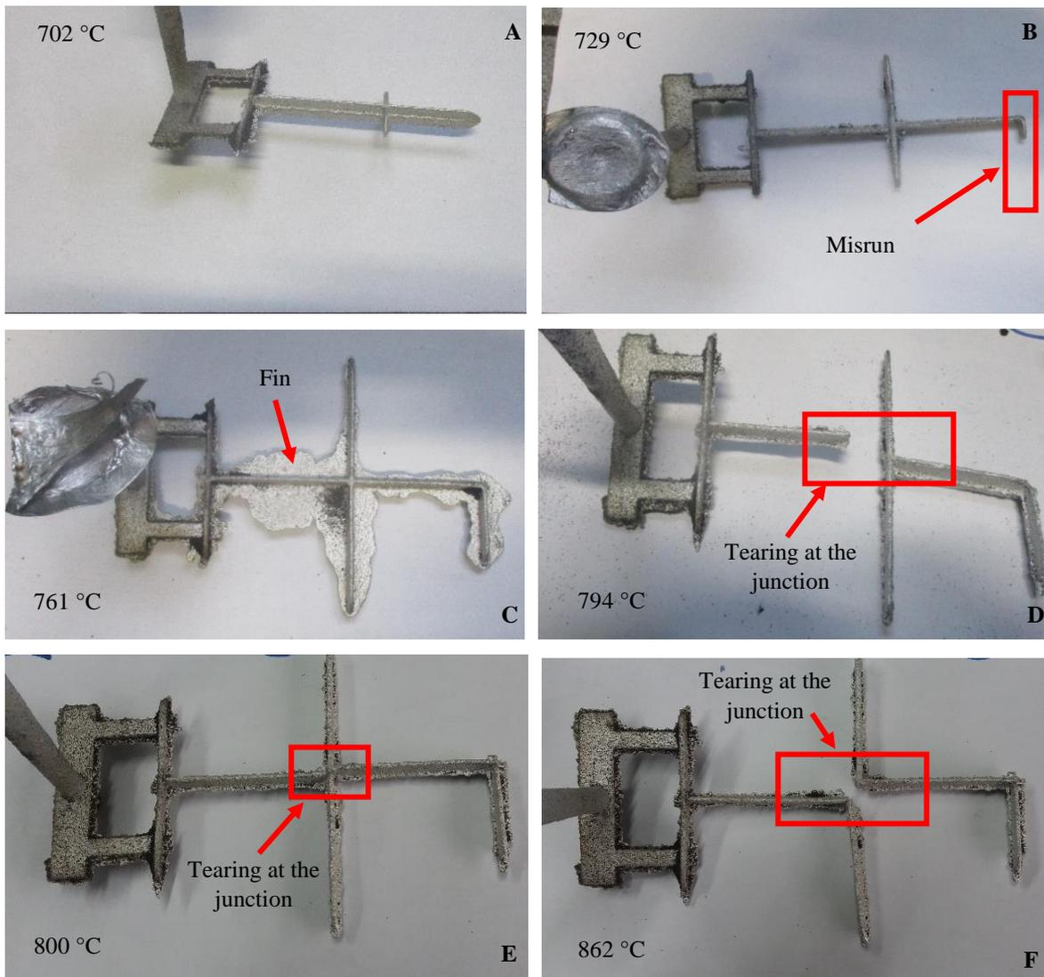
Figure 4. 6: Casting results of 2mm test sample at 702 °C (A), 729 °C (B), 761 °C (C), 794 °C (D), 800 °C (E) and 862 °C (F).
