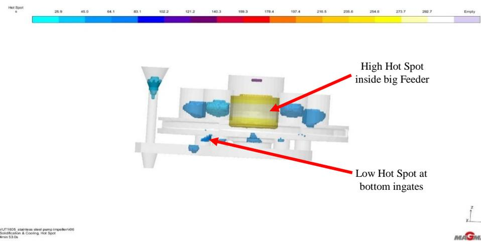
Figure 4. 18: 3D view showing hot spot results at junctions made by bottom ingates and casting.
