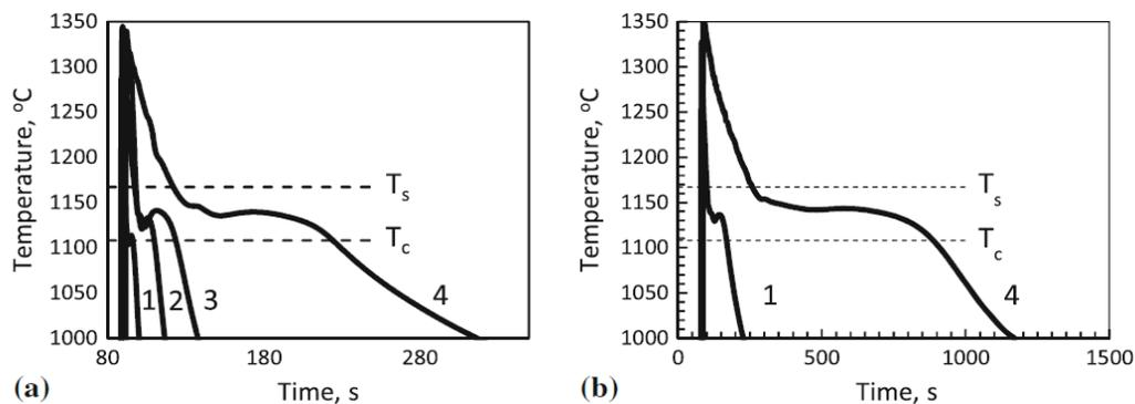
Figure 2. 12: Cooling curves of ductile iron in samples with different wall thicknesses: (a) foundry mould with the silica sand (SMS), (b) foundry mould with the LDADC sand.
