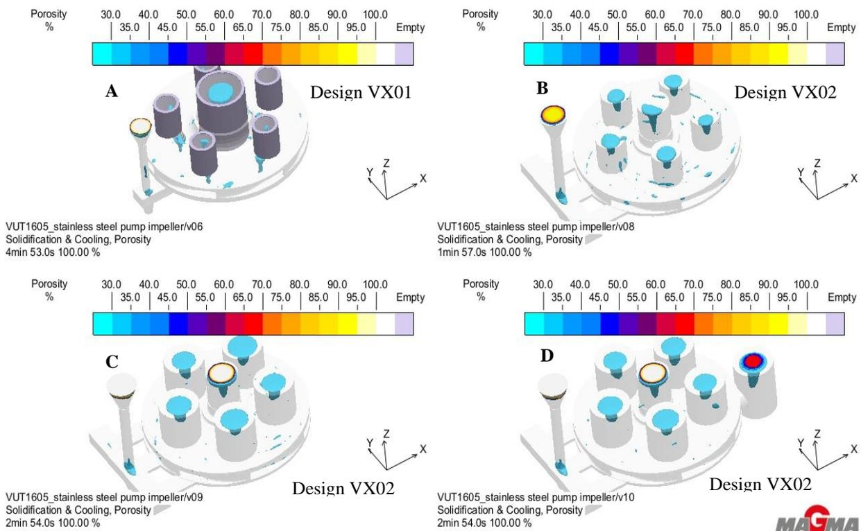
Figure 4. 21: 3D view showing porosity results of different runner system designs
