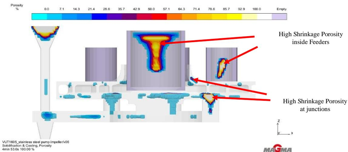
Figure 4. 20: Side-view showing shrinkage porosity at junctions
