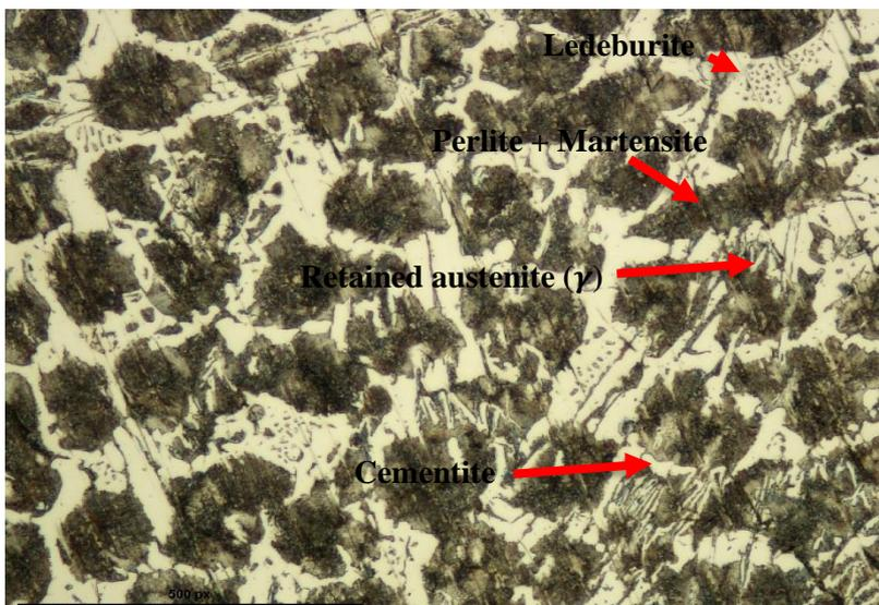
Figure 4. 45: As cast microstructure of a nodular cast iron pump impeller at 500X magnification
