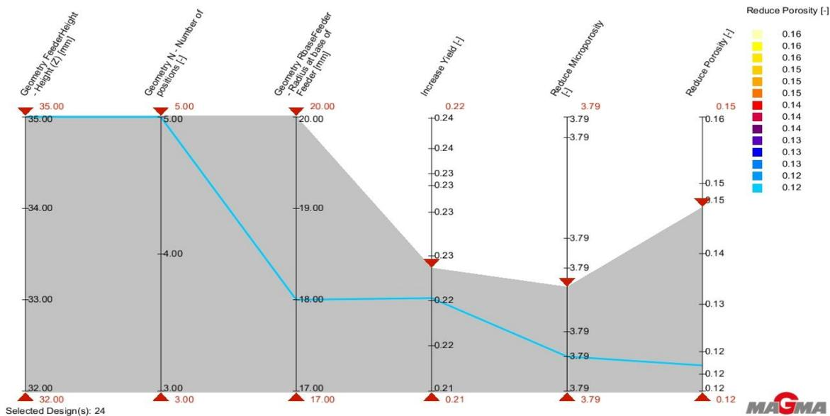
Figure 4. 25: Parallel coordinates results after optimisation simulation (1 best design)
