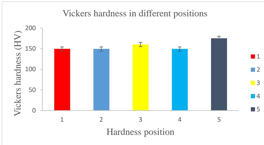
Figure 4. 55: Vickers hardness results of an as cast austenitic stainless steel at different positions
