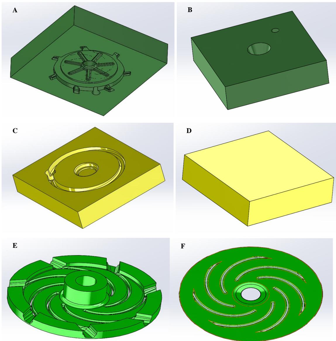
Figure 3. 16: Austenitic stainless-steel moulds cope (A and B), drag (C and D) and core (E and F).
