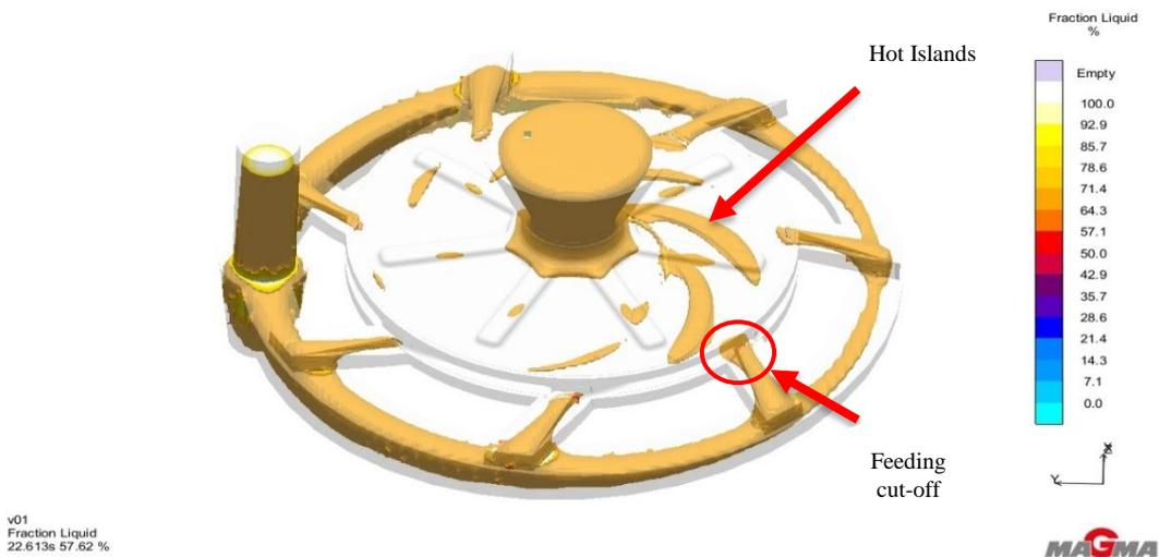
Figure 4. 51: Solidification simulation of design VX04 after 53% solid at 22.6 seconds
