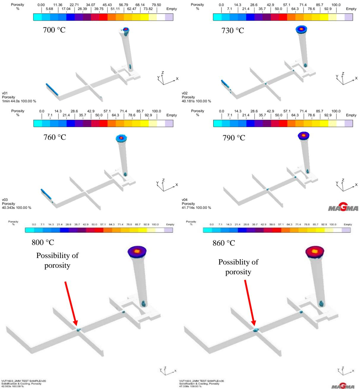
Figure 4.5: Porosity results of 2mm test sample at 700 °C to and 860 °C pouring temperature
