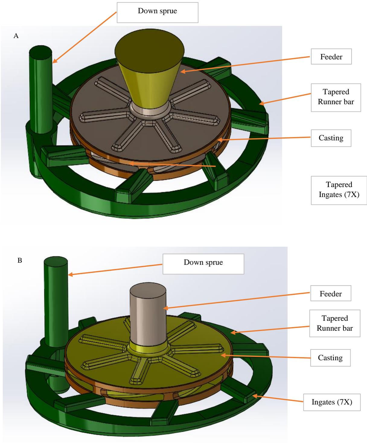
Figure 3. 15: Optimized Design VX04 (A) and Design VX05 (B) runner system.
