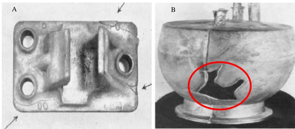
Figure 1. 2: Flow related defects cold-shut (arrowed regions) (A) and misrun (red circle) (B)
