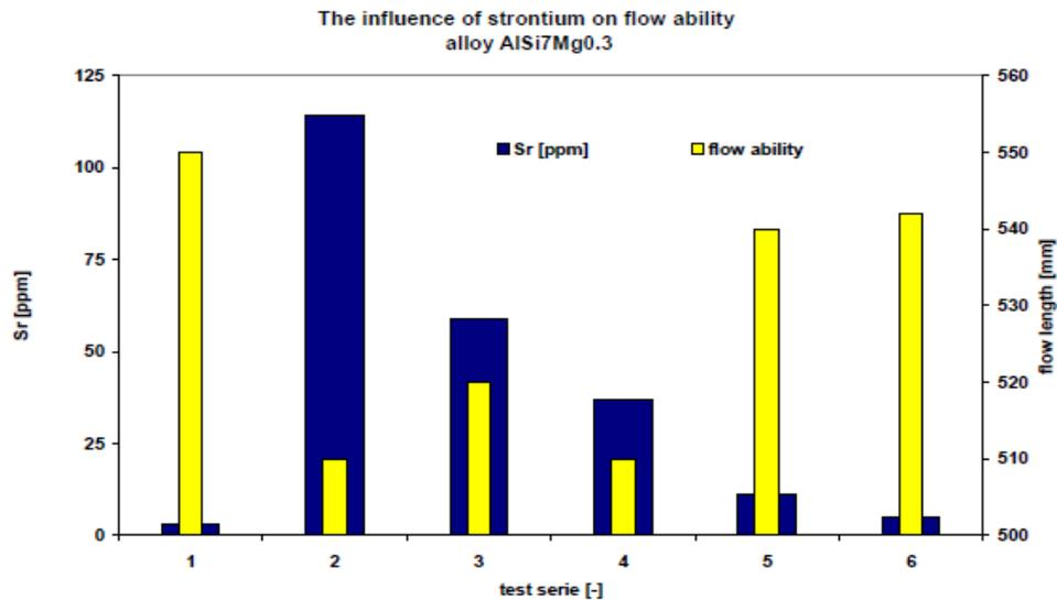
Figure 2. 9: Effect of strontium during solidification process.
