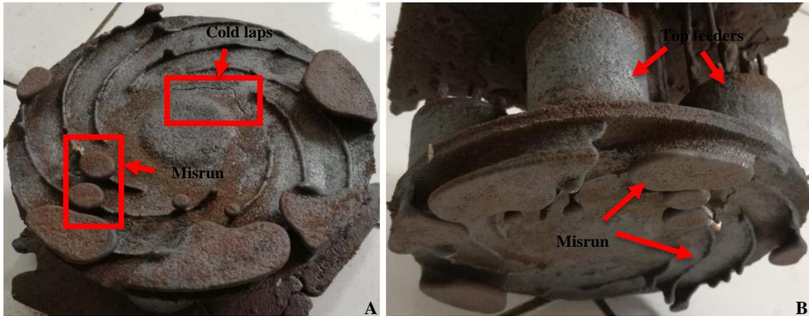
Figure 4. 35A and 4.35B: Defective austenitic stainless-steel pump impeller cast at 1497 °C.
