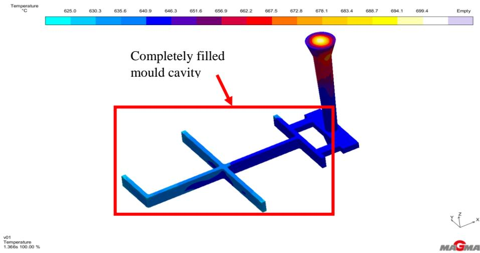
Figure 4. 11: Filling ability of 3 mm test sample at 700 °C pouring temperature
