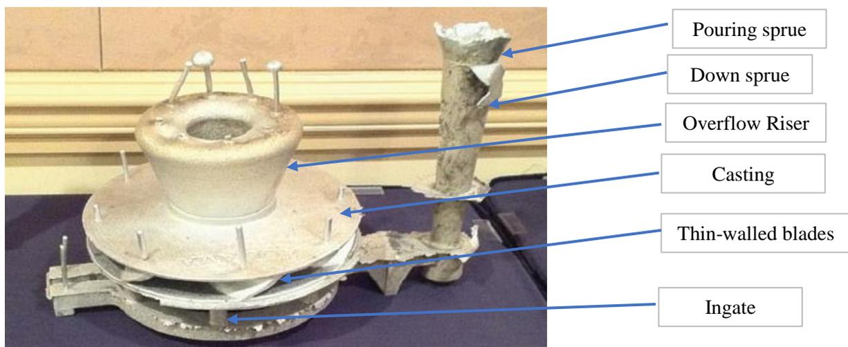
Figure 2. 1: A 3D view of a sand cast with runner system after shake-out.
