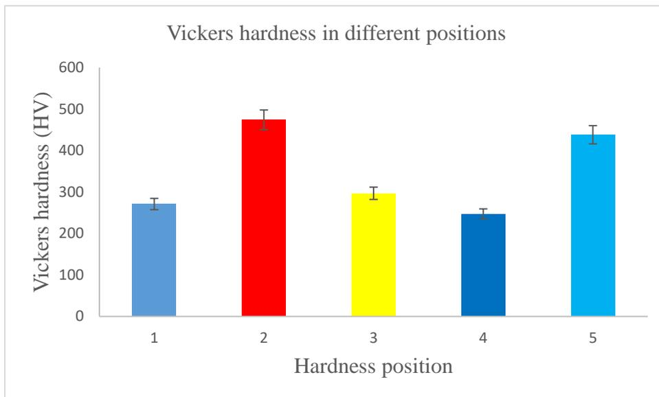
Figure 4. 46: Vickers hardness results of a nodular cast iron pump impeller at different positions
