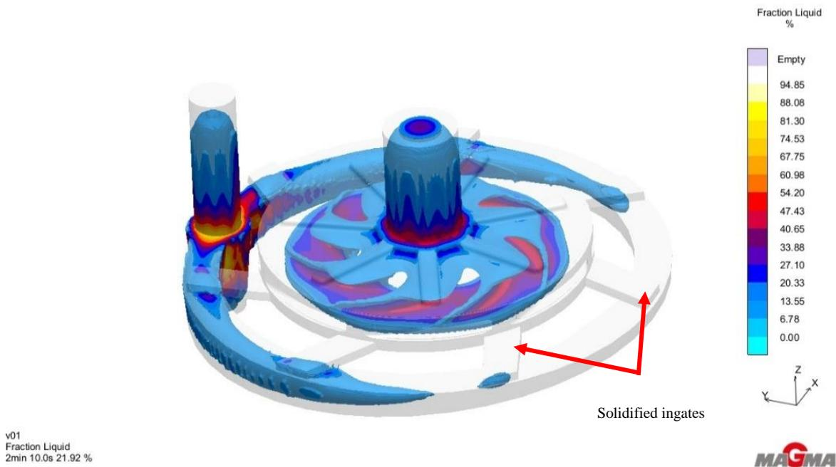
Figure 4. 61: Solidification simulation of design VX05 after 78.1% solid in 130 seconds
