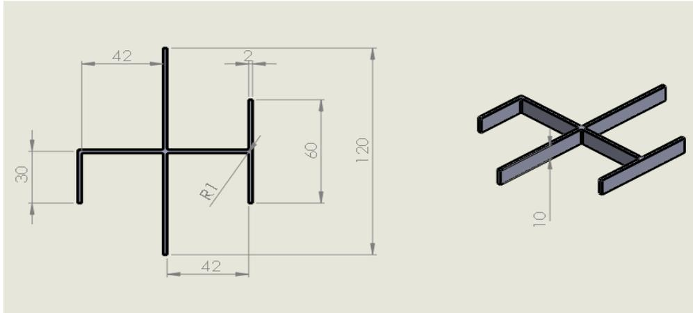
Figure 3. 1: A schematic representation of the 2mm test sample showing different junction geometries.
