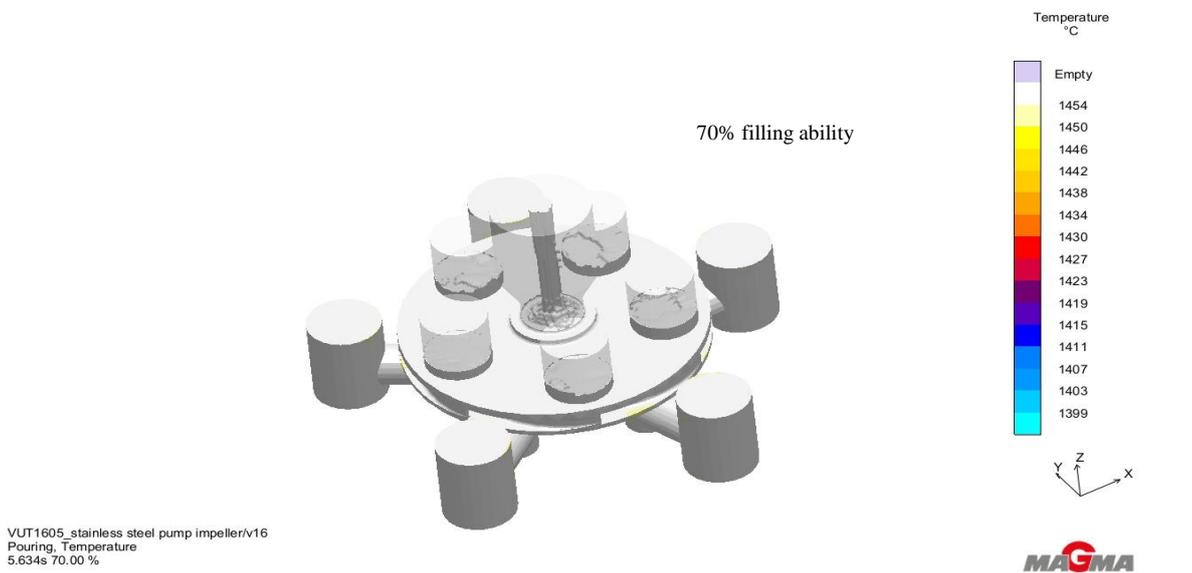
Figure 4. 32: Filling simulation of the casting after 5.6 seconds
