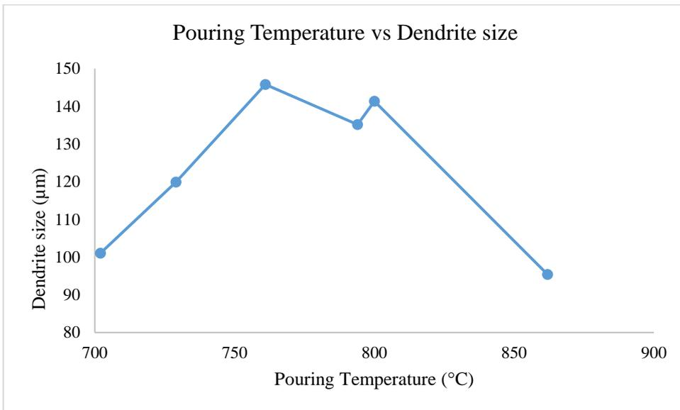
Figure 4. 7: Relationship between pouring temperature and grain size.
