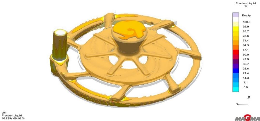
Figure 4. 50: Solidification simulation of design VX04 after 31% solid at 16.7 seconds
