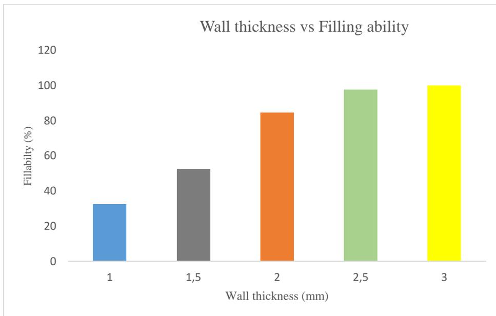
Figure 4. 12: Wall thickness vs filling ability at 700°C pouring temperature
