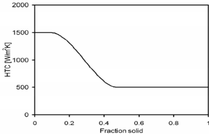
Figure 2. 14: Heat Transfer Coefficient (HTC) as a function of the solid fraction in the surface of the casting next to the mould.
