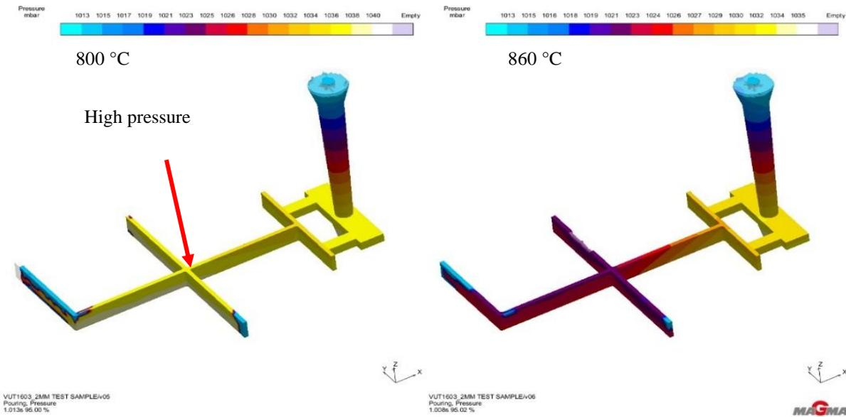
Figure 5.3C: A representation of metal pressure after 1.1 seconds of 2 mm test sample at 700 °C to 860°C pouring temperature.
