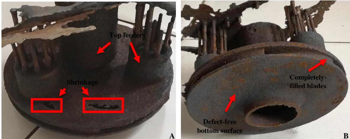
Figure 4. 44A and 4.44B: Completely-filled nodular cast iron pump impeller with minor shrinkage defects cast at 1501 °C.
