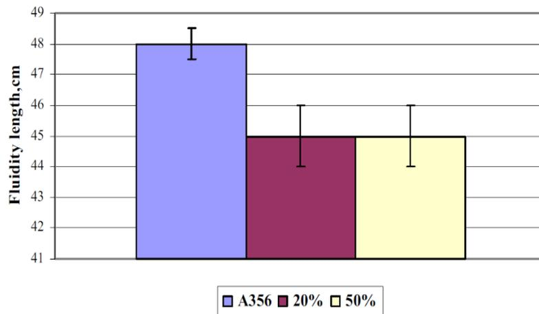
Figure 2. 5: Effect of scrap quantity on the fluidity measurements of three different alloys: Aluminium A356 with no scrap addition, aluminium A356 + 20 % scrap addition, aluminium A356 + 50 % scrap addition.
