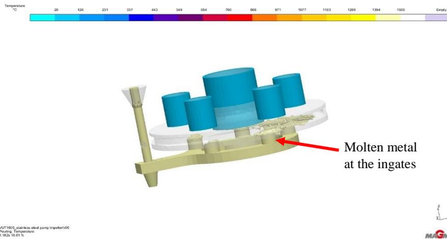
Figure 4. 17: Filling simulation of design VX 01
