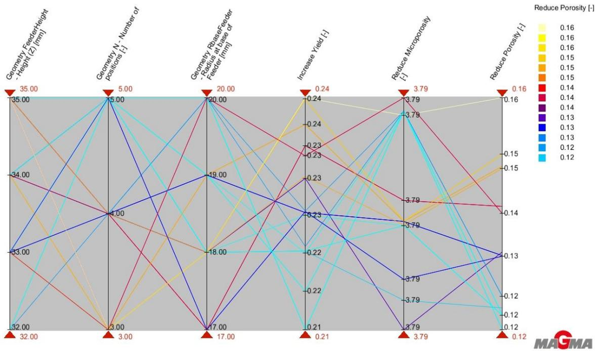
Figure 4. 23: Parallel coordinates results after optimisation simulation (30 different designs)
