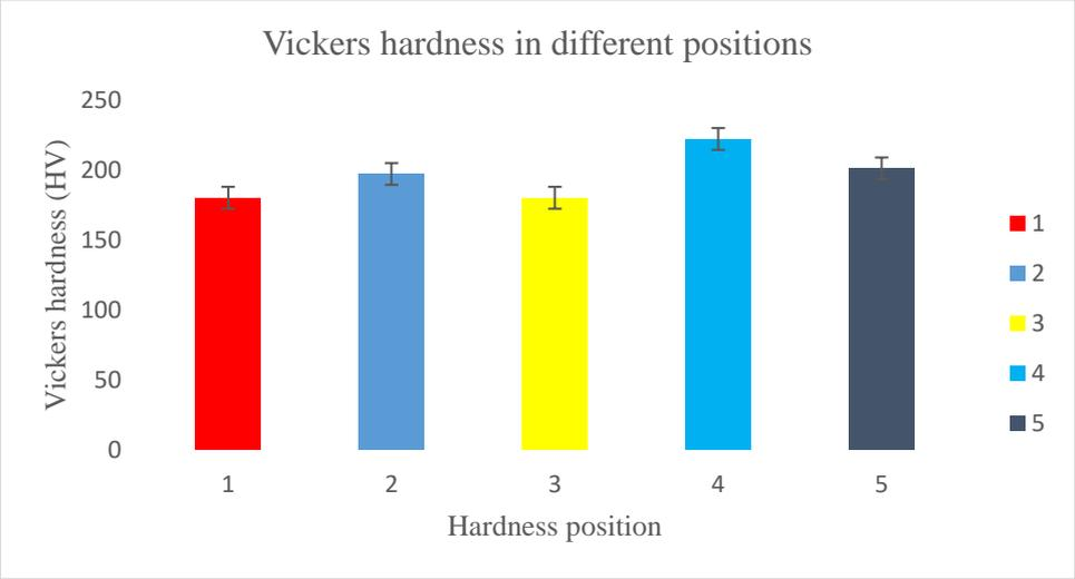
Figure 4. 66: Vickers hardness results of a nodular cast iron pump impeller at different positions
