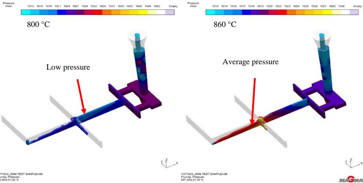
Figure 4.3B: Metal pressure after 640 milliseconds of 2 mm test sample at 700 °C to 860 °C pouring temperature.
