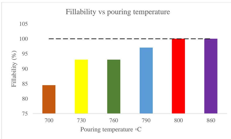
Figure 4. 2: Pouring temperature vs filling ability percentage
