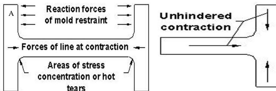
Figure 1. 3: Schematic representation of contraction stresses distribution in an I section (A) and T section (B)
