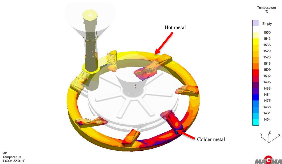
Figure 4. 47: Filling simulation of design VX04 at 32 % filling ability
