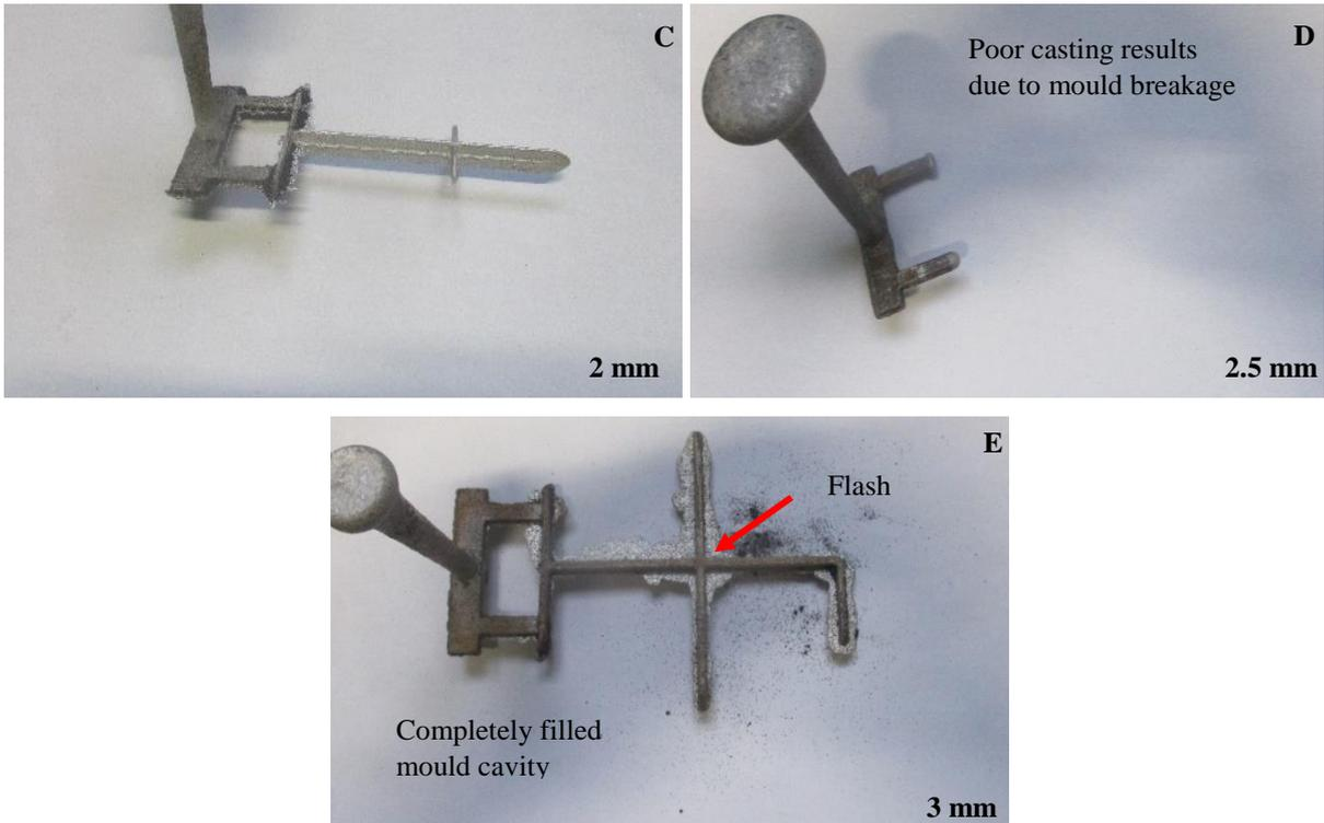
Figure 4. 13: Casting results at 700 °C of 1 mm test sample(A), 1.5 mm (B), 2 mm (C), 2.5 mm (D) and 3 mm (E).
