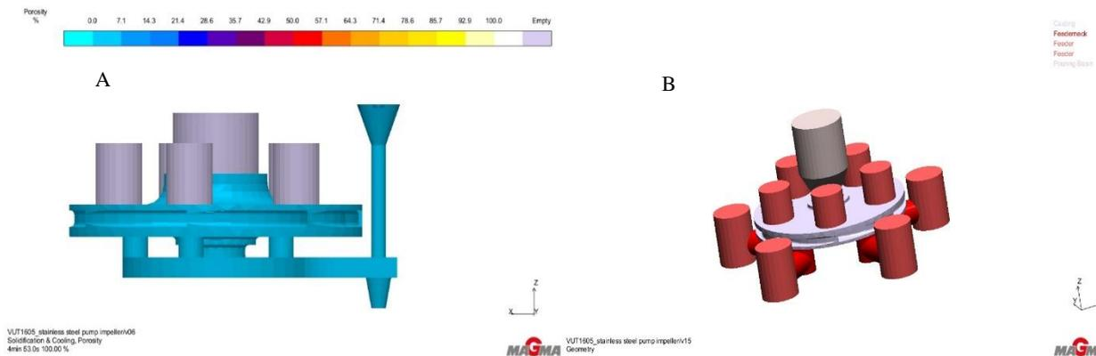
Figure 3. 11: Design VX01 (A) vs design VX02 (B)
