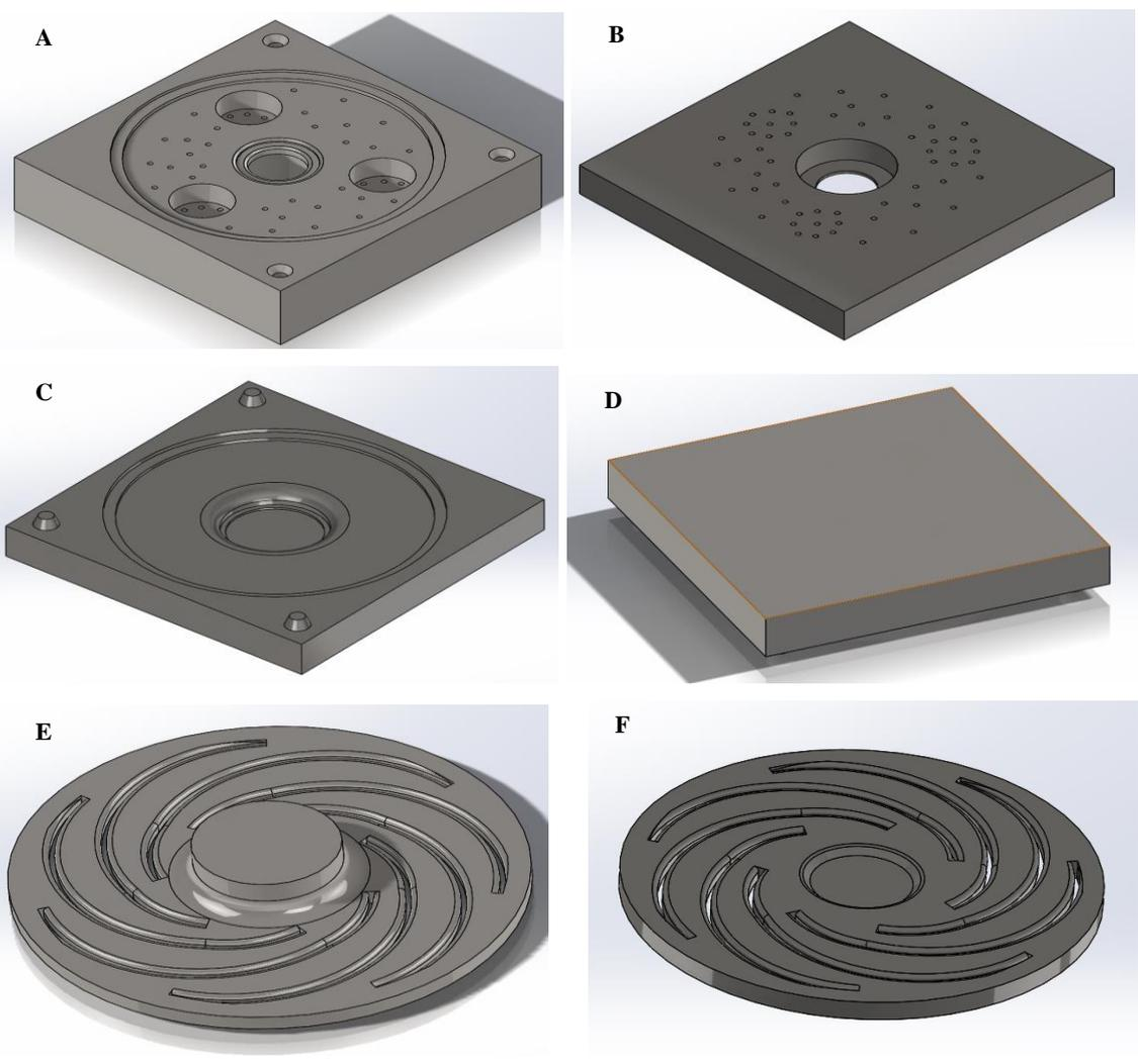
Figure 3. 13: Nodular cast iron moulds cope (A and B), drag (C and D) and core (E and F).
