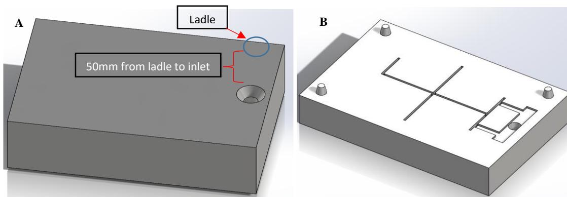
Figure 3. 9: 3D view cope (A) and drag (B) of test sample mould
