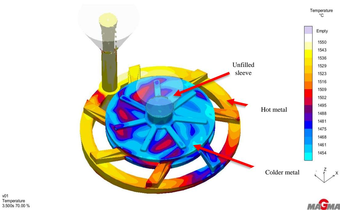
Figure 4. 49: Filling simulation of design VX04 at 70% filling ability
