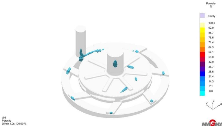
Figure 4. 62: Porosity results of design VX05 after 2100 seconds solidification
