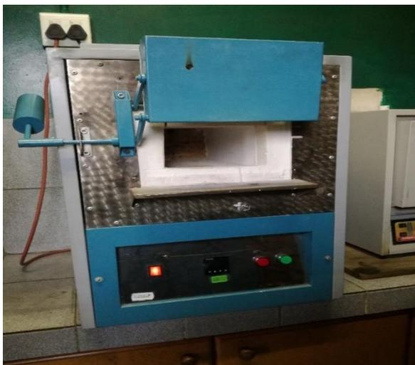
Figure 3. 3: Overview of Muffle furnace
