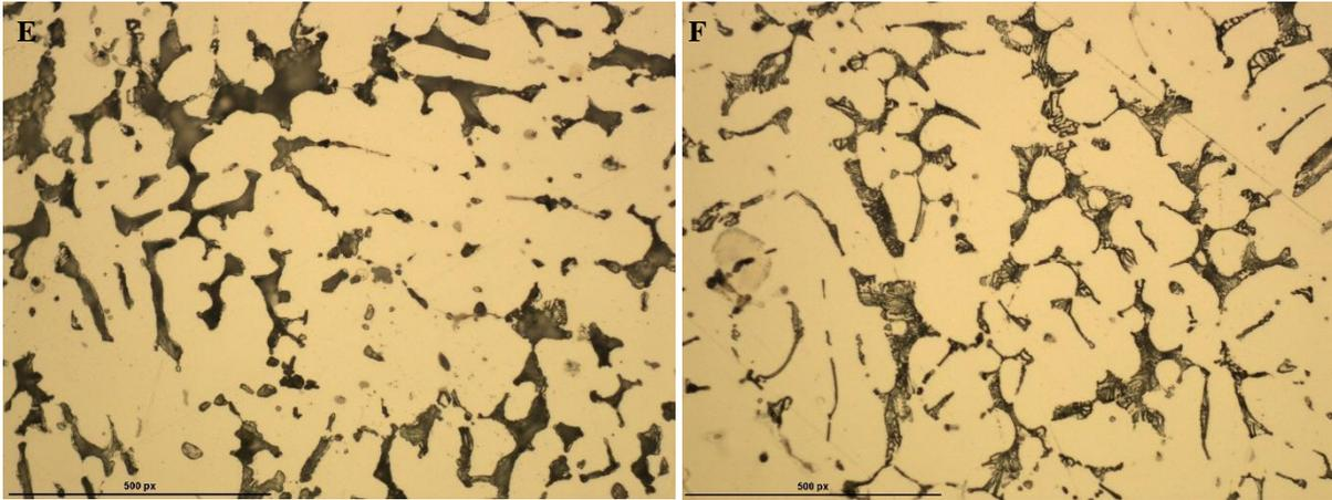
Figure 4. 8: Microstructural results of 2mm test sample at different pouring temperatures at 50X magnification.
