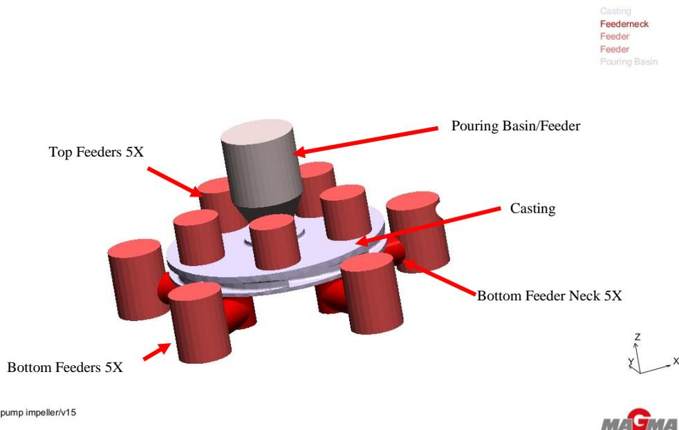
VUT1605\_stainless steel pump impeller/v15
