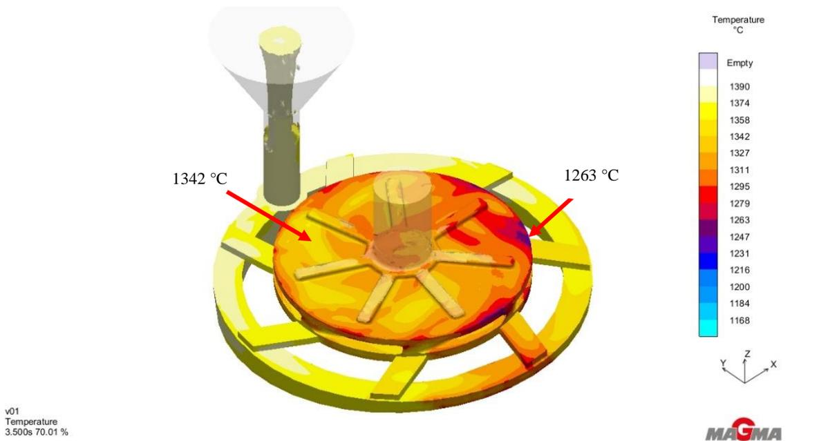
Figure 4. 58: Filling simulation of design VX05 at 70.01% filling ability after 3.5 seconds
