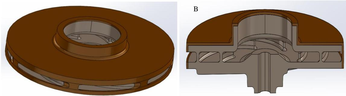
Figure 3. 10: 3D view (A) and section view (B) of a pump impeller
