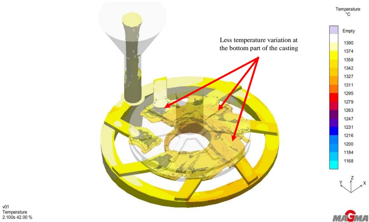
Figure 4. 57: Filling simulation of design VX05 at 42% filling ability after 2.1 seconds
