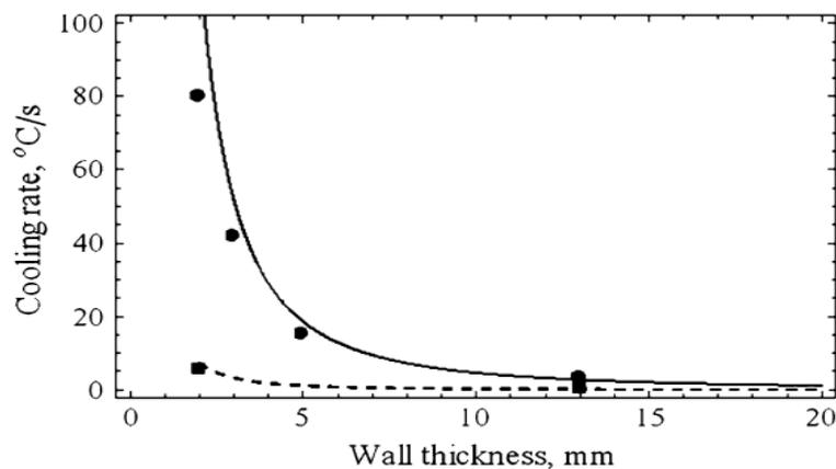
Figure 2. 13: Effect of wall thickness on the cooling rate of the casting: solid curve represents experimental points for SMS mould, dotted curve represents experimental points for LDASC mould.
