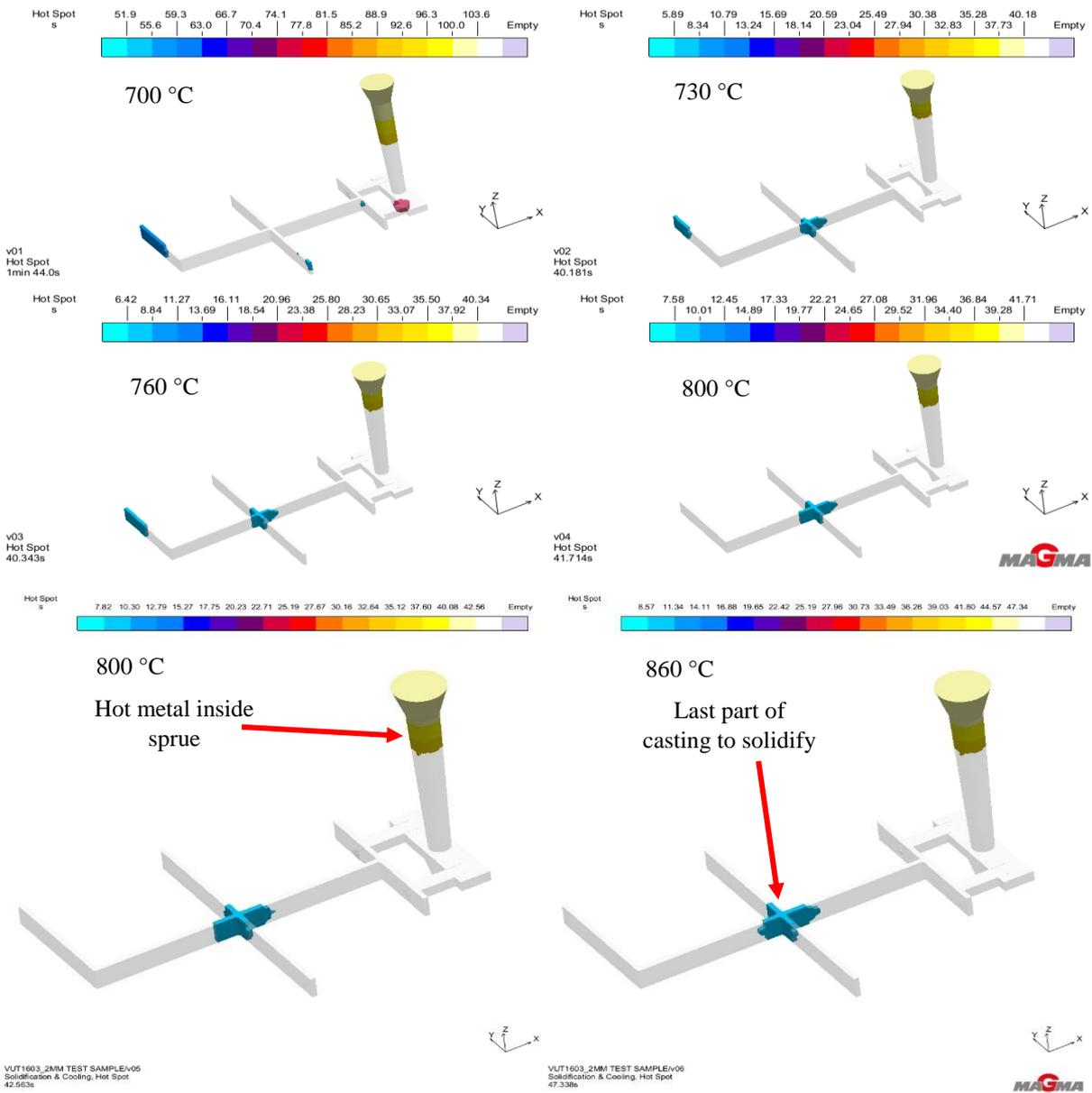
Figure 4.4: Hot Spot results of 2 mm test sample at 700 °C to 860 °C pouring temperature.
