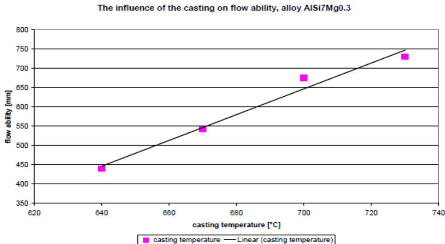
Figure 2. 4: The influence of the pouring temperature on flowability of an aluminium AlSi7Mg<sub>0.3</sub> alloy.
