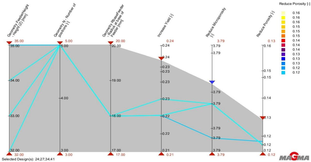
Figure 4. 24: Parallel coordinates results after optimisation simulation (4 best designs)
