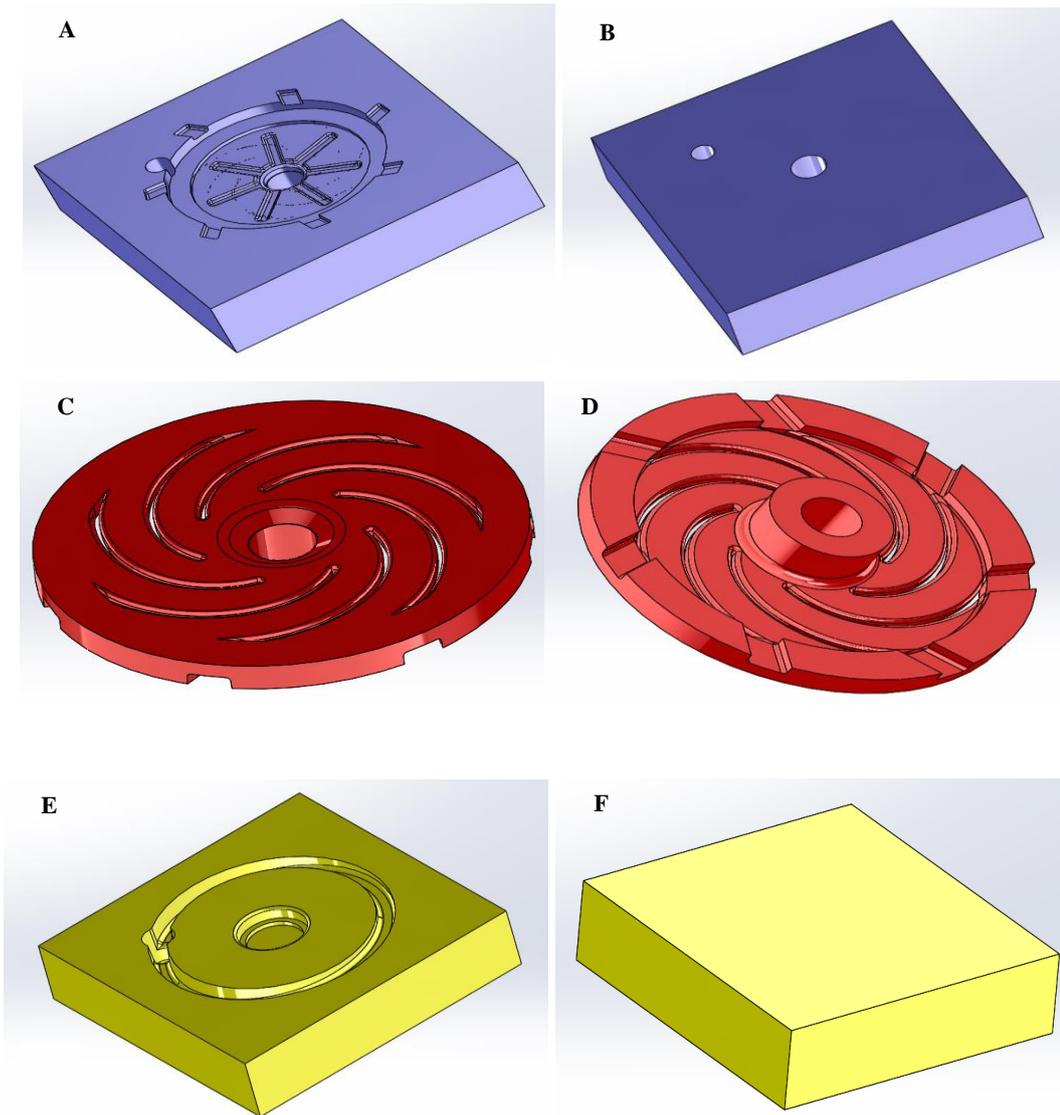
Figure 3. 17: Nodular cast iron moulds cope (A and B), drag (C and D) and core (E and F).
