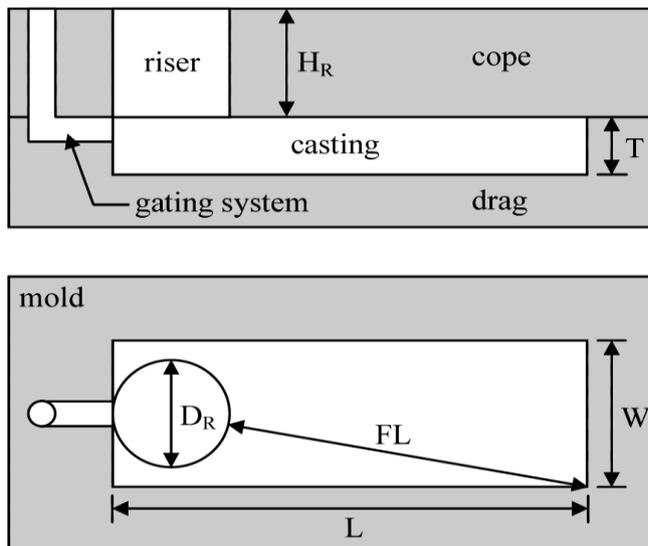
Figure 1. 4: A schematic representation of the feeding distance (FD)
