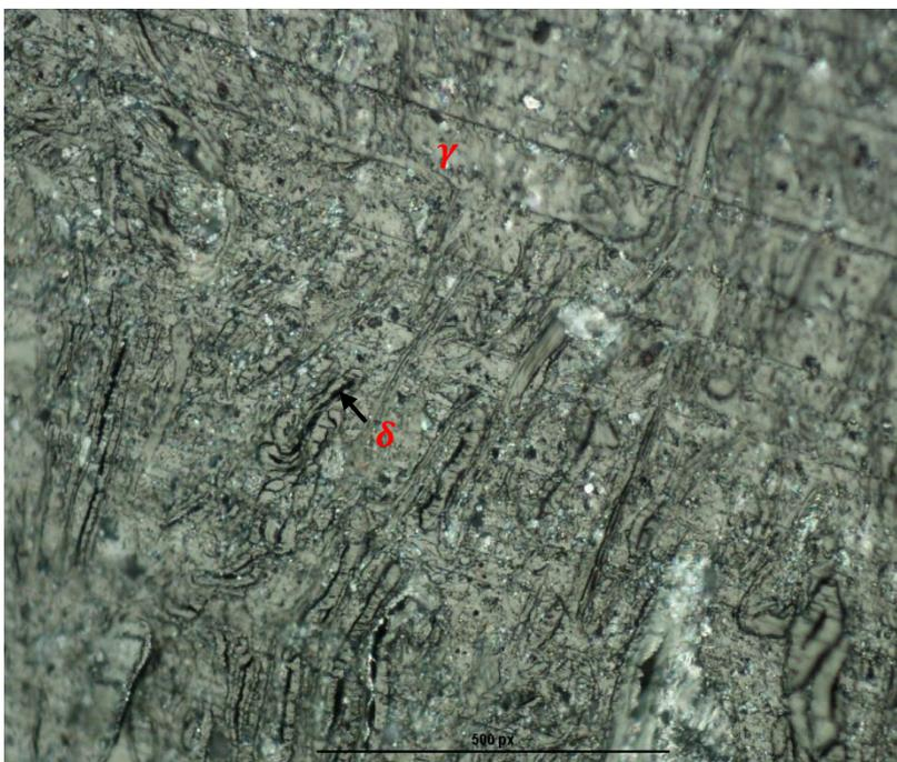
Figure 4. 36: As cast microstructure of an austenitic stainless steel pump impeller at 50X magnification
