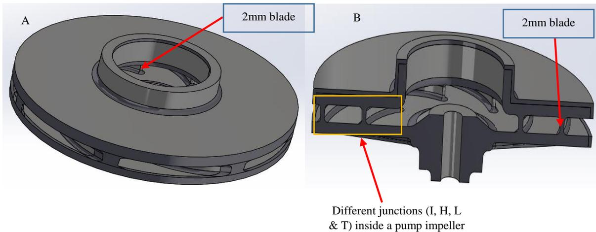
Figure 1. 1: Thin-walled (2mm) blades inside pump impeller, isometric view (A) section view (B)
