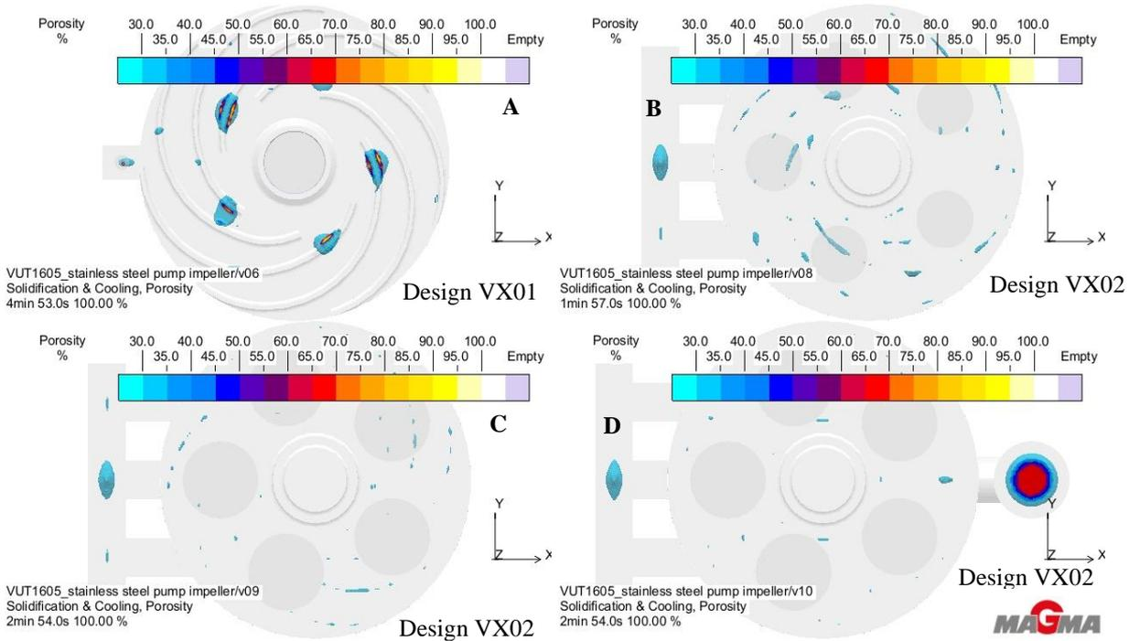
Figure 4. 22: Top view showing porosity results of different runner system designs
