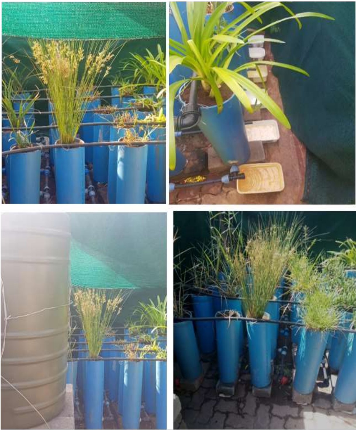
Figure 3.2: Experimental setup (nursery-based type setup vegetated biofilter), 2020
