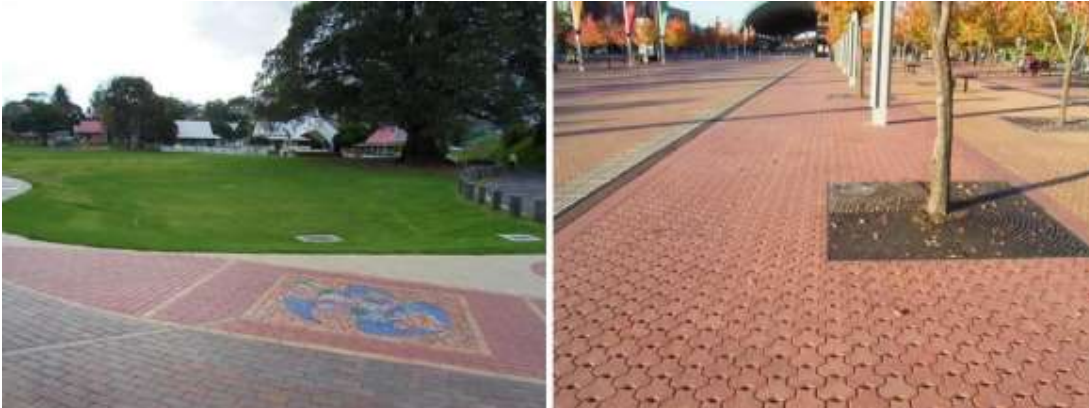
Figure 2.4: Permeable Pavements (WSUD, 2011)
