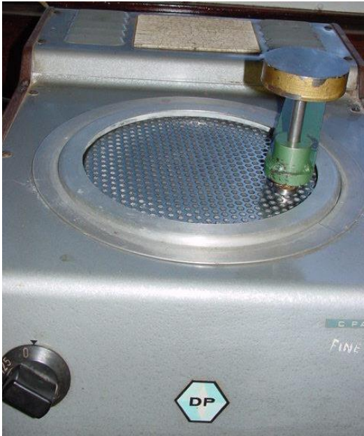
Figure 3.2: Test rig used in laboratory for pin-on-disk tests
